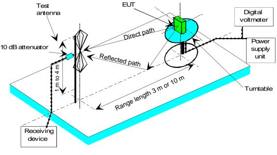
Typical measuring arrangement common for ground plane test sites is presented in figure B.4.
