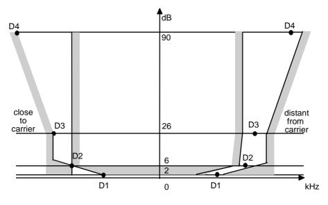
Figure A.1: IF filter characteristics
