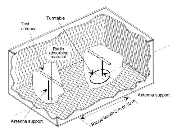
Figure B.1: A typical anechoic chamber
