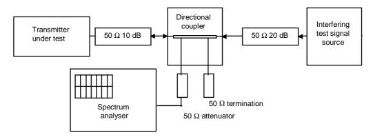
Figure 3: Measurement arrangement
