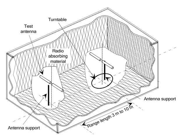
Figure B.1: A typical anechoic chamber
