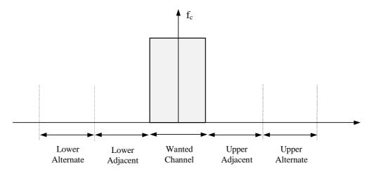
Figure 1: Adjacent and alternate channel definitions
