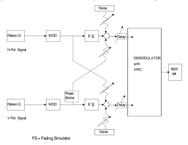
Figure A.1: Measurement test set
