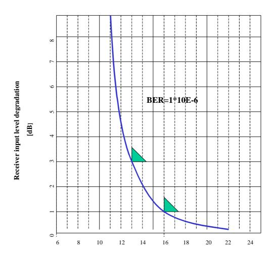
Figure B.3: Co-channel "internal" digital interference sensitivity limits in cross-polar application (referred to point B')
