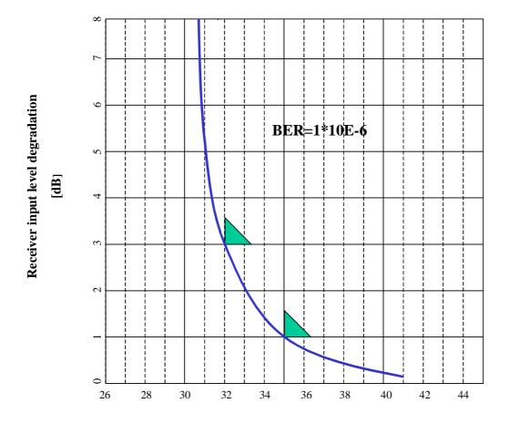
Figure B.1: Co-channel digital "external" interference sensitivity mask
