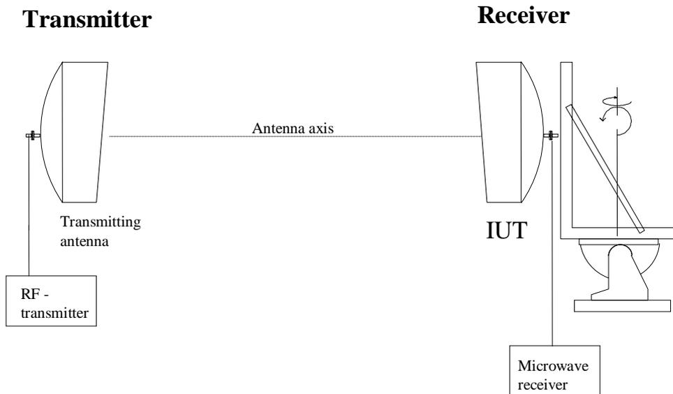
**Figure 2: Example of arrangement for the measurement of the radiation pattern in the azimuth plane**
