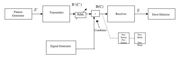
Figure 15: Test configuration for CW spurious interference
