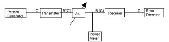
Figure 14: Test configuration for background BER
