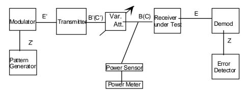
Figure 12: Test configuration for dynamic level range
