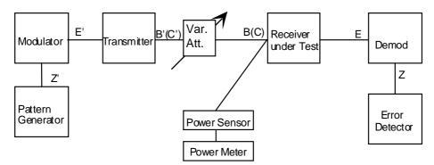
Figure 11: Test configuration for input level range
