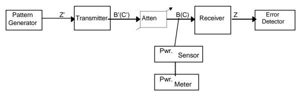
Figure 11: Test configuration for BER as a function of RSL
