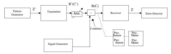
Figure 14: Test configuration for CW spurious interference
