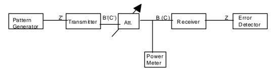
Figure 12: Test configuration for background BER
