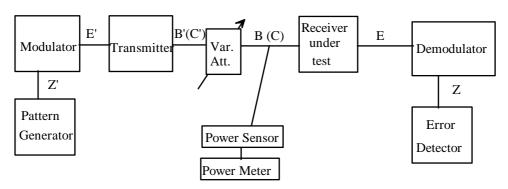
Figure 9: Test Configuration for input level range
