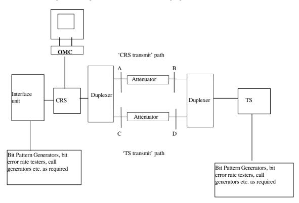
NOTE: TDD systems may only require a single path with one attenuator.
