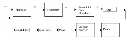
Figure 8: Test Configuration for conducted antenna port spurious emissions
