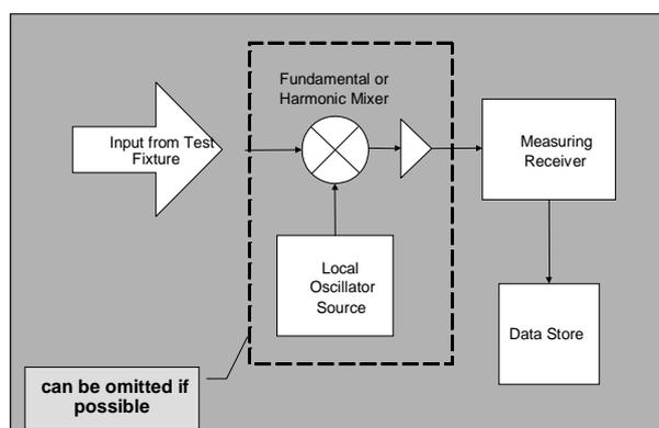
Figure 7: Principal test setup for measuring spurious emissions above 40 GHz
