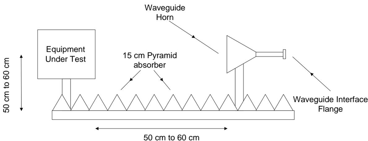
Figure 1: Test fixture
