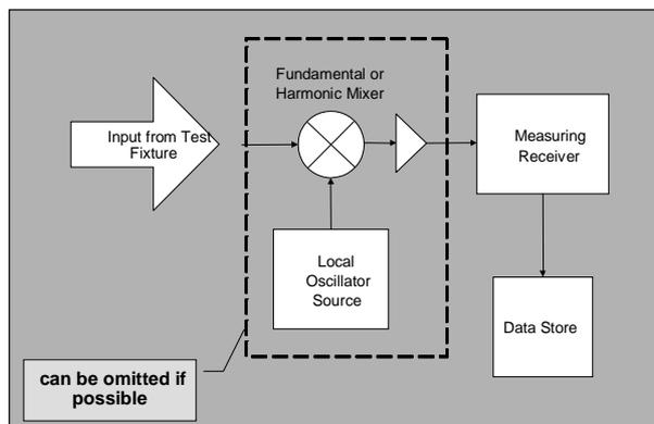
**Figure 4: Principal test set-up for mean power (e.i.r.p) measurements of transmitter operating in the 76 GHz to 77 GHz band**
