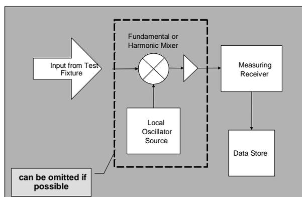
**Figure 5: Principal Test setup for measuring out of band radiation above 40 GHz**
