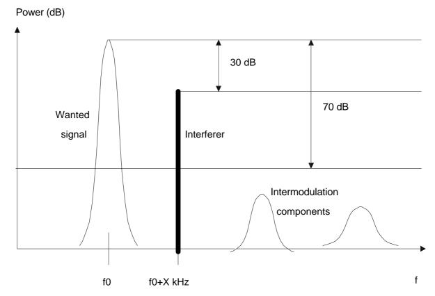
Figure 5: Example of TX intermodulation attenuation
