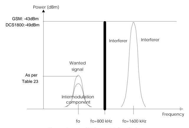
Figure 6: Example of RX intermodulation rejection
