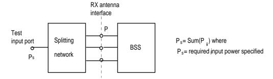
Figure 1a: Receiver test setup
