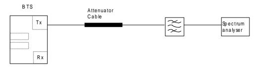
Figure B.4: Test set-up for Intra Base station Intermodulation Attenuation (6.8.) TX-Band
