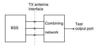
Figure 1b: Transmitter test setup
