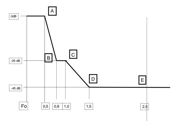
Figure 3: DS-CDMA spectrum mask normalized to channel spacing
