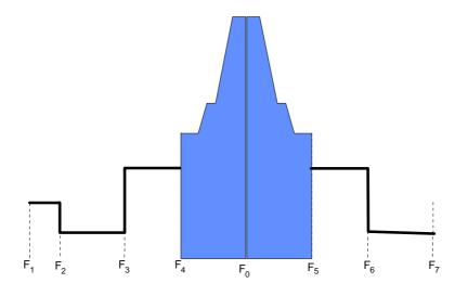
Figure 4: Spectrum mask for transmitter spurious emissions
