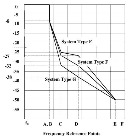
Figure 4: Power spectrum masks for system type E, F and G (fo = actual carrier frequency)
