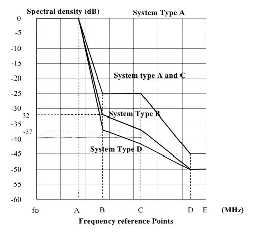
Figure 3: Power spectrum masks for system type A, B, C and D (fo = actual carrier frequency)
