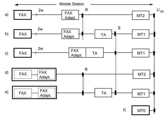
Figure 2/03.45: Reference configurations
