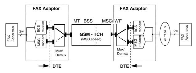
Figure 6/03.45: Fax Adaptor working principle
