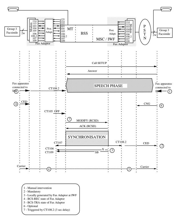
Fig. II-7b/03.45 - Mobile Originated Call - Speech then Fax (Data Call Direction is Mobile
