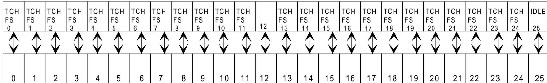
Figure 7a: TDMA frame mapping for TCH/FS + SACCH/FS
