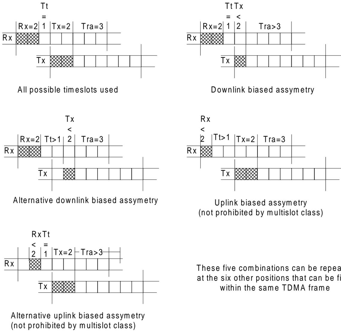
These five combinations can be repeated at the six other positions that can be fitted within the same TDMA frame
