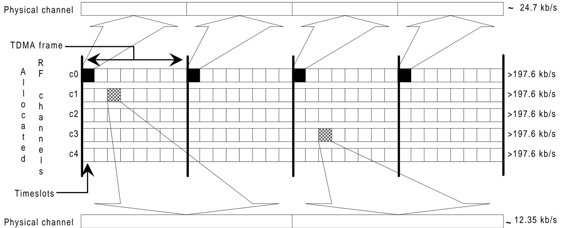
(This example of a physical channel is hopping using 3 of every other TDMA frame)
