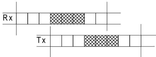
This configuration could be used for HSCSD or GPRS
