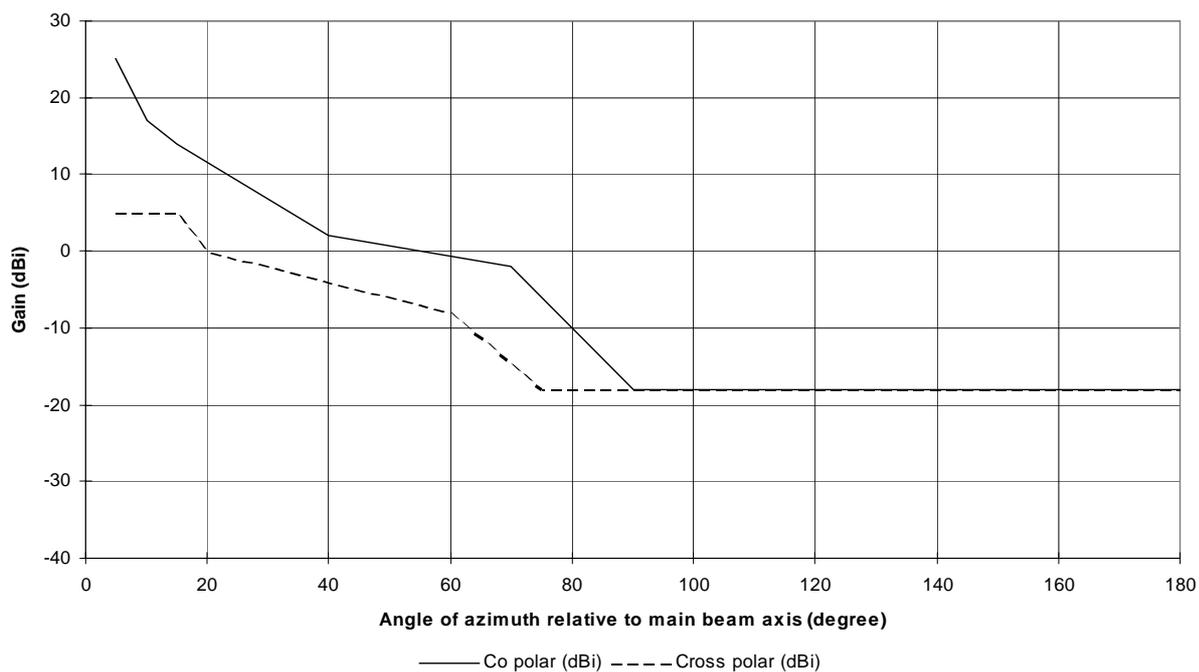
Figure 7b: RPEs for class 2 antennas in the frequency range 6
