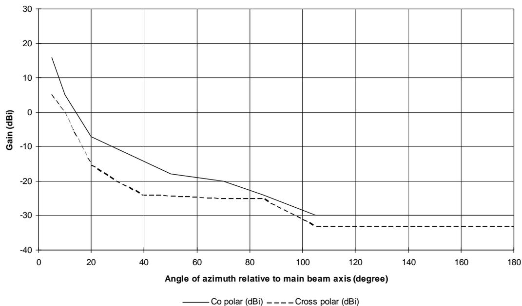
Figure 2d: RPEs for class 4 antennas in the frequency range 1
