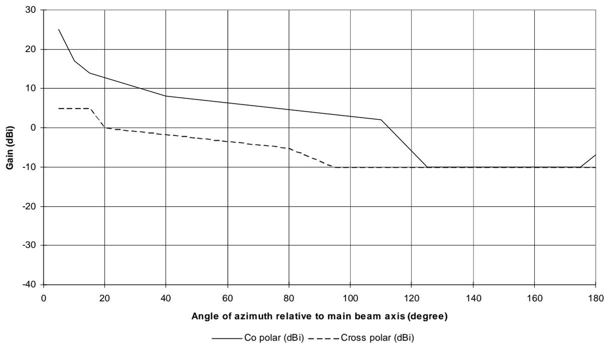
Figure 7a: RPEs for class 1 antennas in the frequency range 6
