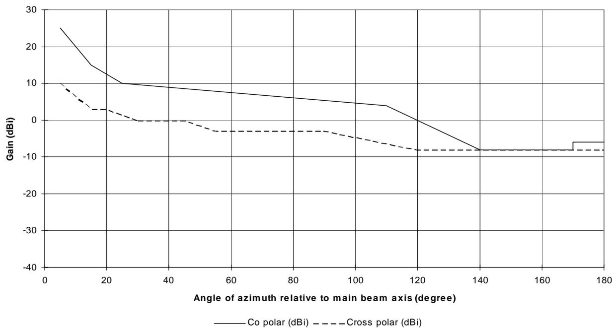
Figure 3a: RPEs for class 1 antennas in the frequency range 2
