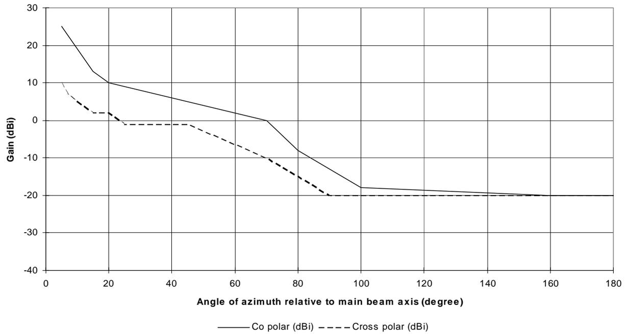
Figure 3b: RPEs for class 2 antennas in the frequency range 2
