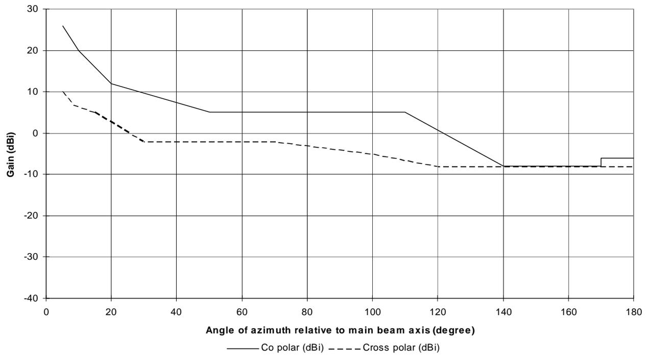
Figure 2a: RPEs for class 1 antennas in the frequency range 1
