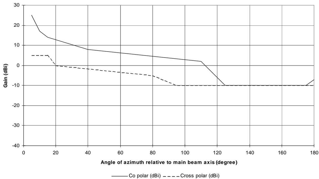
Figure 6a: RPEs for class 1 antennas in the frequency range 5
