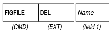
Figure 32: FIGFILE DEL message structure
