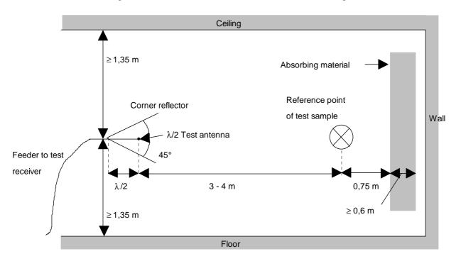
Figure A.2: Indoor site arrangement (shown for horizontal polarization)
