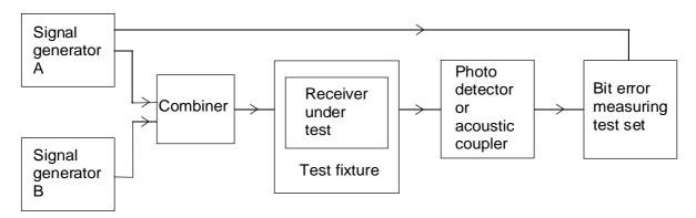
Figure 8: Measurement arrangement - adjacent channel selectivity
