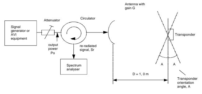
Figure 11: Measurement arrangement - transponder sensitivity
