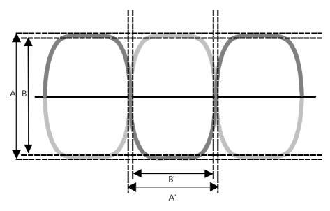
Figure 3: Eye pattern measurement
