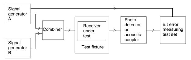
Figure 9: Measurement arrangement - spurious response rejection
