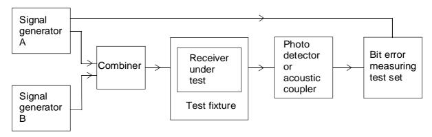
Figure 7: Measurement arrangement - co-channel rejection
