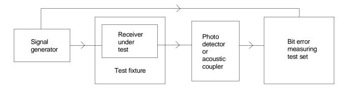
Figure 2: Measuring arrangement for calibration
