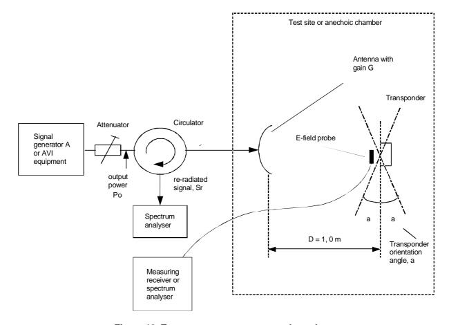
Figure 12: Test arrangement - transponder wake up
