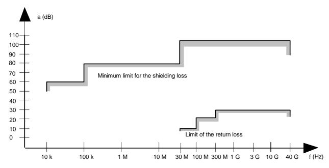
Figure A.3: Specification for shielding and reflections
