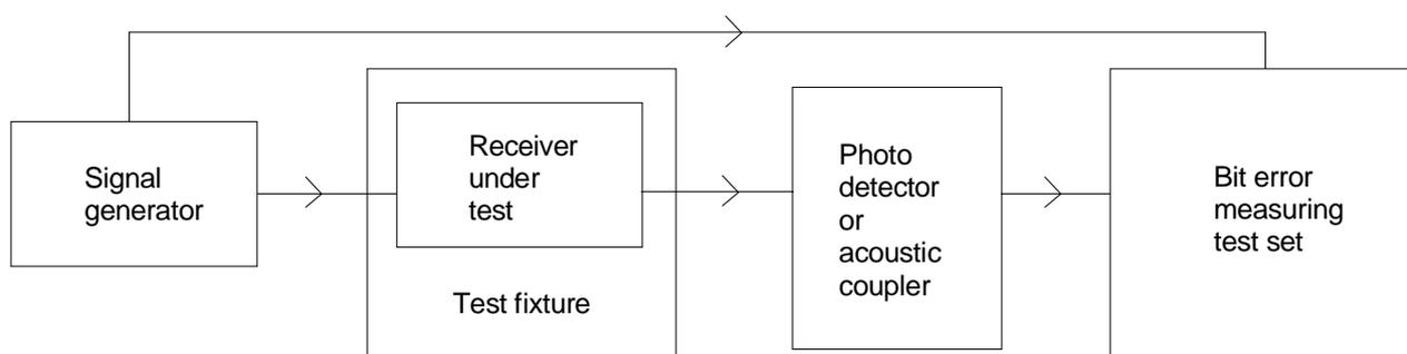
**Figure 2: Measuring arrangement for calibration**
