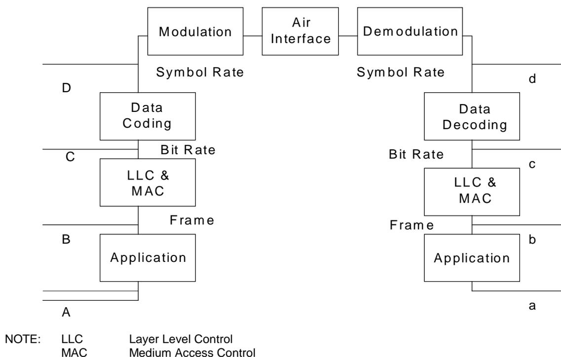
**Figure 1: Measuring points for data stream measurements**
