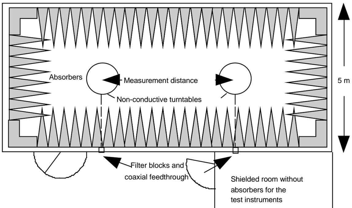
Figure A.4: Example of construction of an anechoic shielded chamber
