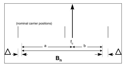
Figure E.6: Maximum value of nominated bandwidth for Case (iii), a ≠ b
