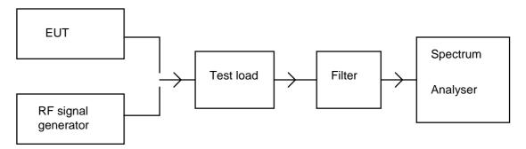
Figure D.1: Measurement arrangement for conducted emissions
