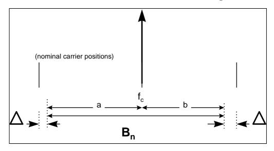
Figure E.5: Maximum value of nominated bandwidth for case (iii), a = b
