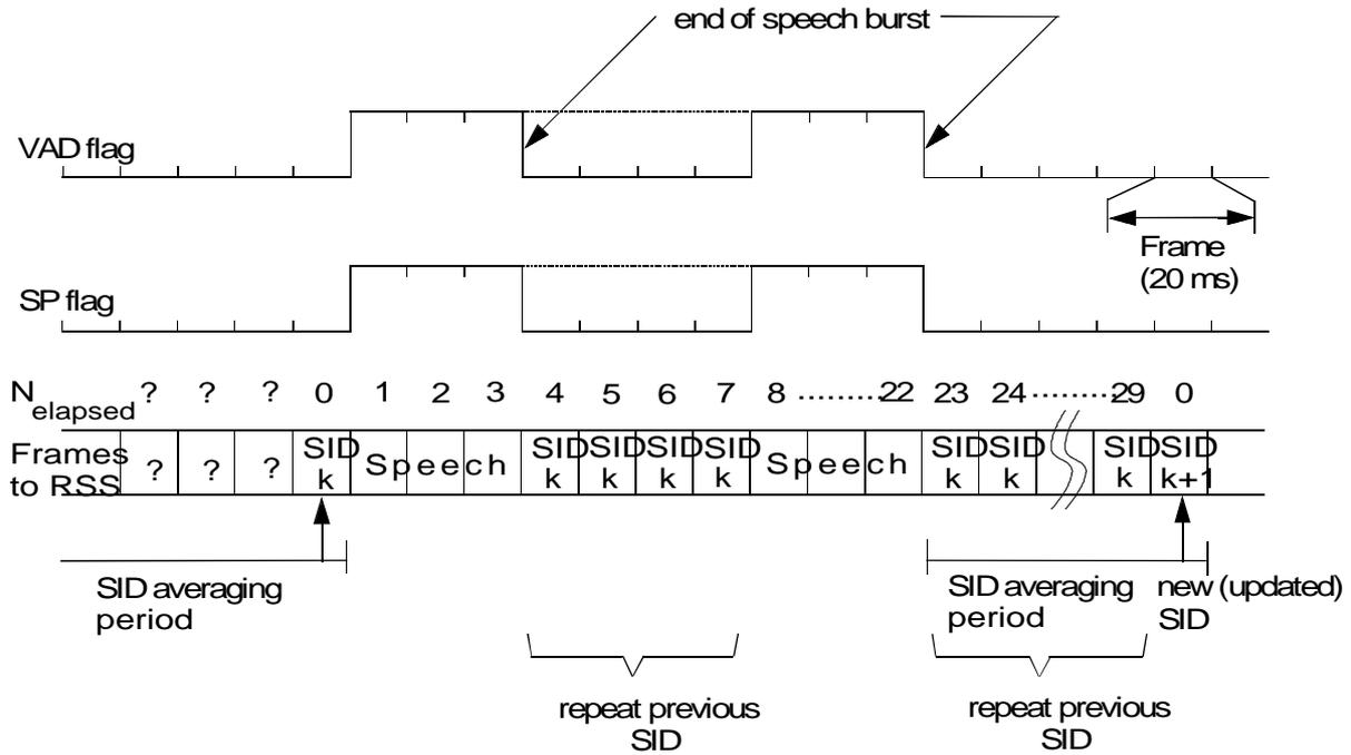
Figure 3: Handling of short speech bursts ( $N_{elapsed} < 24$ ) (Example)
