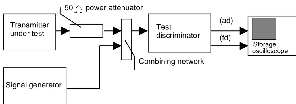
**Figure 3: Measurement arrangement**
