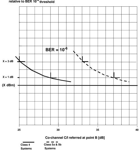
Receiver Input Level at Reference Point C relative to BER 10<sup>-6</sup> threshold
