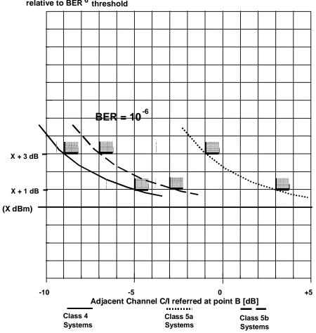
Receiver Input Level at Reference Point C relative to BER<sup>-6</sup> threshold
