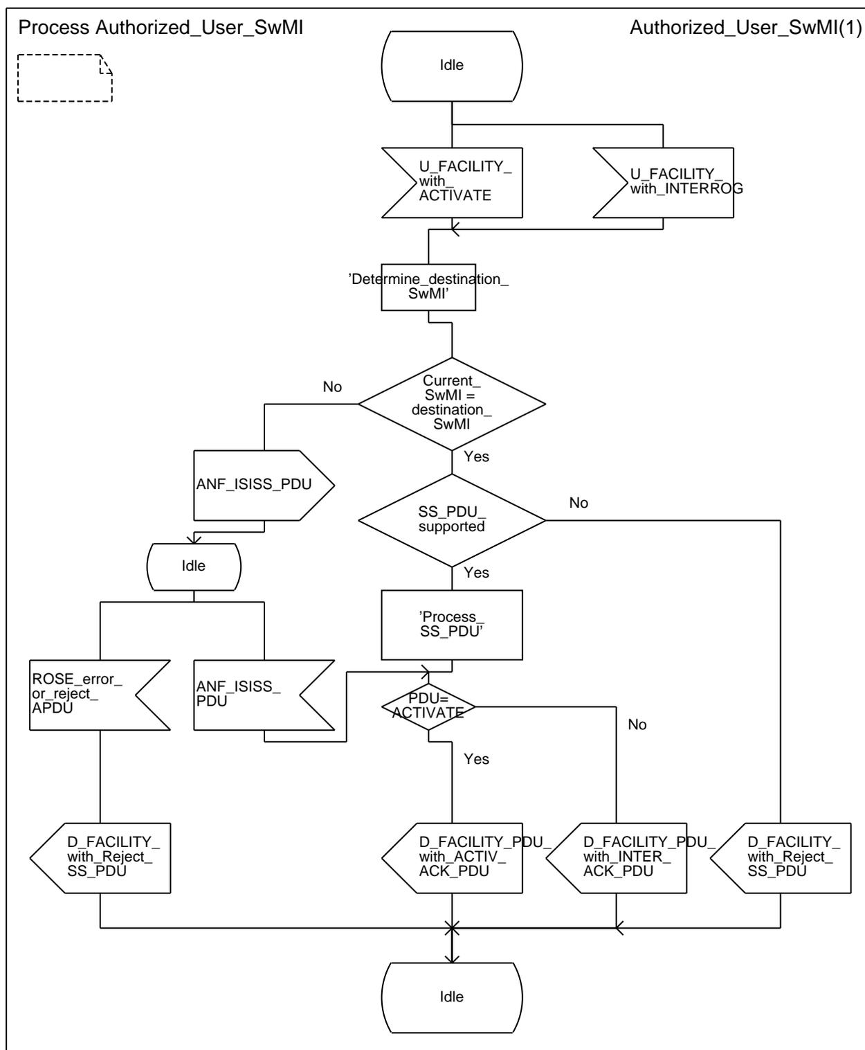
NOTE: This SDL diagram is the generic supplementary service activation; in the case of SS-DL, additional activation/activation ack flows from/to the authorized user home SwMI to/from the monitored user home SwMI are to be taken into account.
