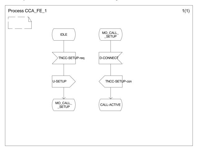
Figure 4: Process description for CCA to which FE1 is collocated
