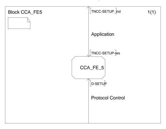
Figure 13: Service interaction for CCA to which FE5 is collocated
