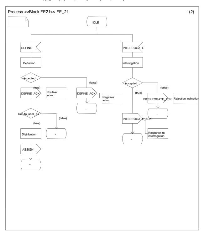
Figure 6: Process description for FE21 state IDLE
