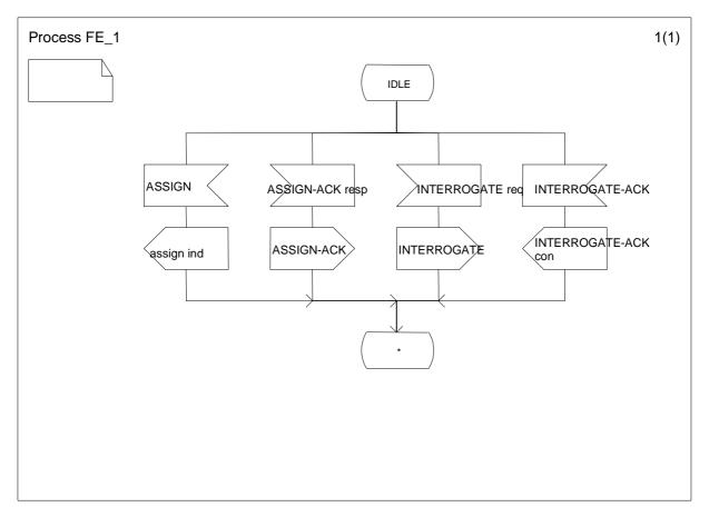
Figure 2: Process description for FE1
