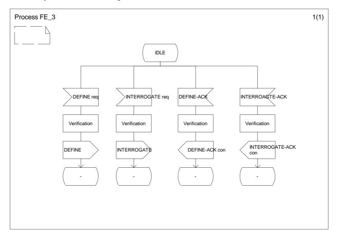
Figure 10: Process description for FE3
