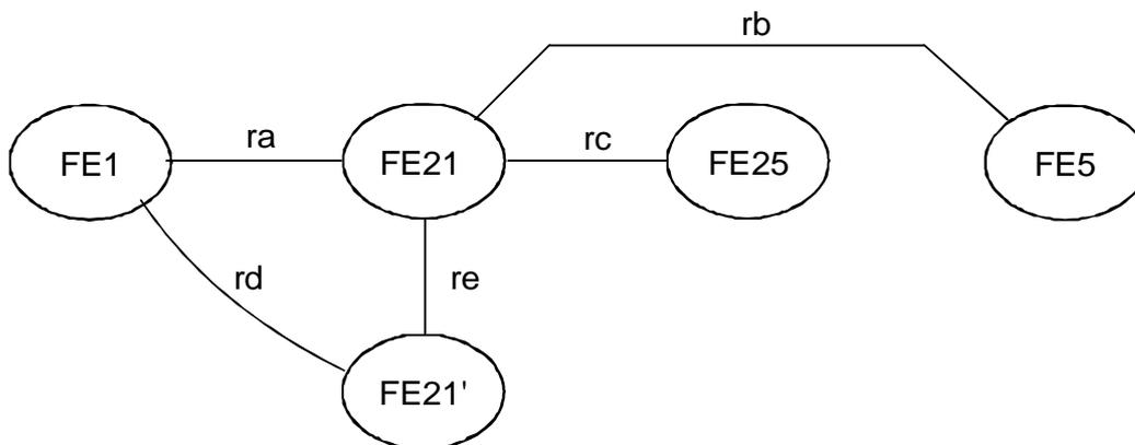
**Figure 2: Functional model for the operational part of SS-HOLD with location change of the served user**
