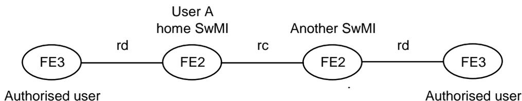
**Figure 2: Functional model for the management part of SS-CAD**
