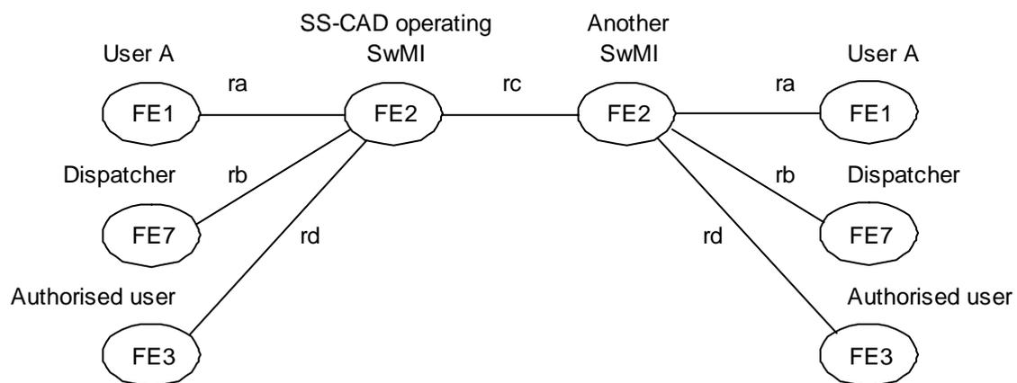
**Figure 1: Functional model for the operational part of SS-CAD**
