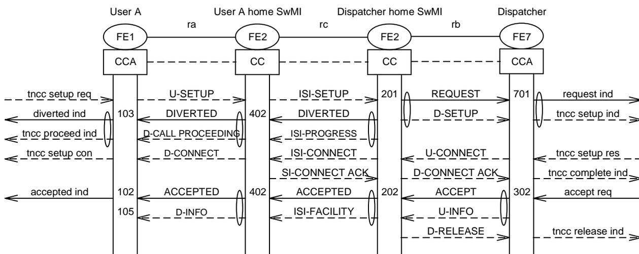
Figure 15: Authorization in called user SwMI when dispatcher is in that SwMI
