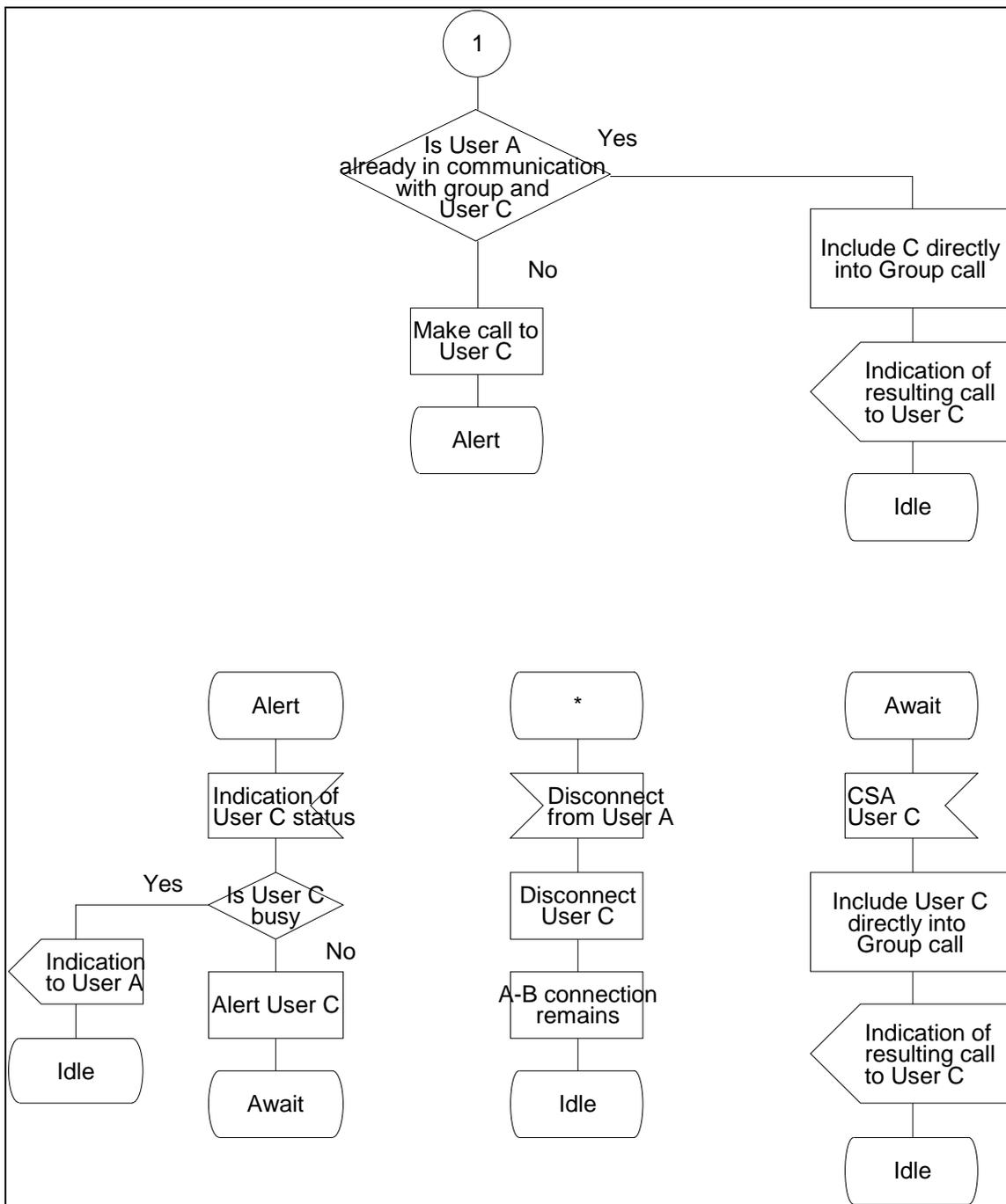
Figure 2: Sheet 2 of 2, SS IC, overall SDL
