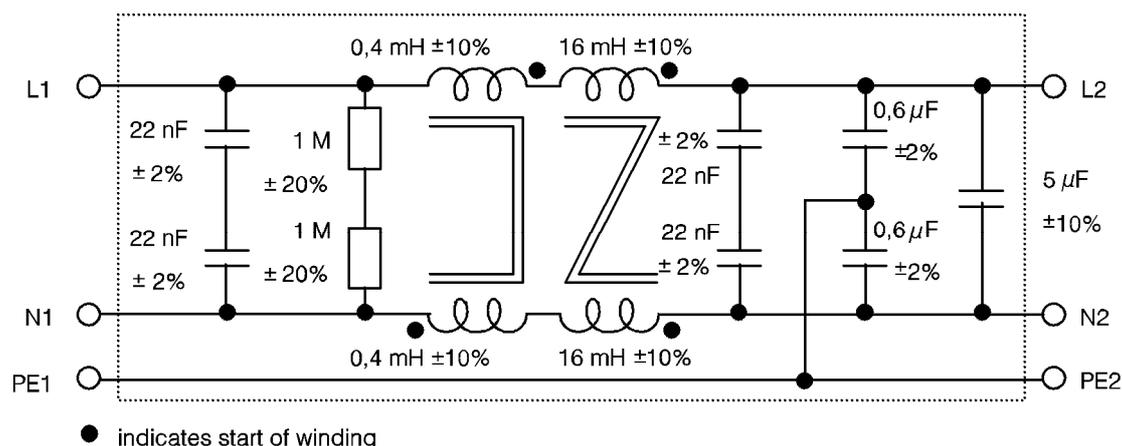
NOTE: The impedance matching network is required to protect the mains supply and the power source for remote power feeding from test overvoltages and to establish standard termination conditions for the test. It is used:
