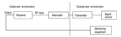
Figure 5: Test configuration for receivers
