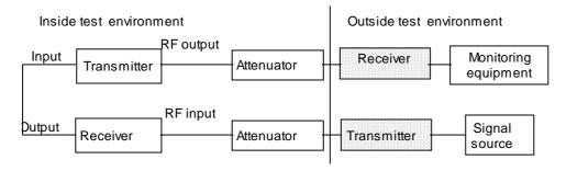
Figure 6: Test configuration of transceivers
