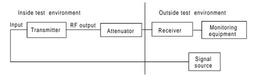
Figure 4: Test configuration for transmitters
