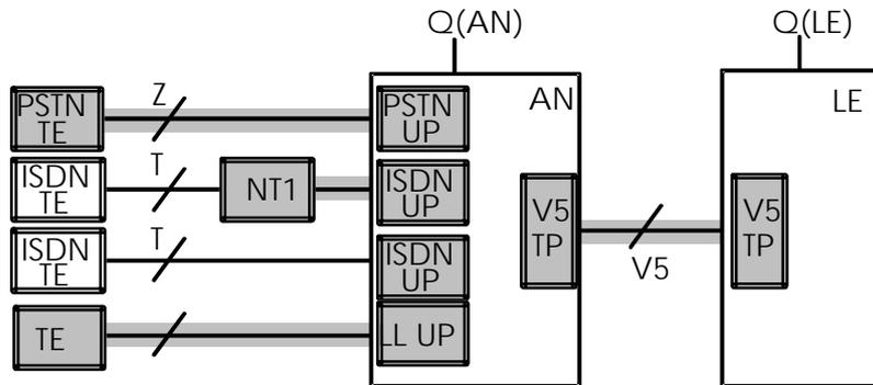
NOTE: Shaded areas are subject to V5 fault and performance management. User ports represent the different configurations for Line Circuit (LC), Line Termination (LT), Exchange Termination (ET) and Network Termination (NT) as indicated in EN 300 324-1 [4] and EN 300 347-1 [5]. For leased lines (semi-permanent lines), the present document only covers aspects which are common to PSTN and ISDN.
