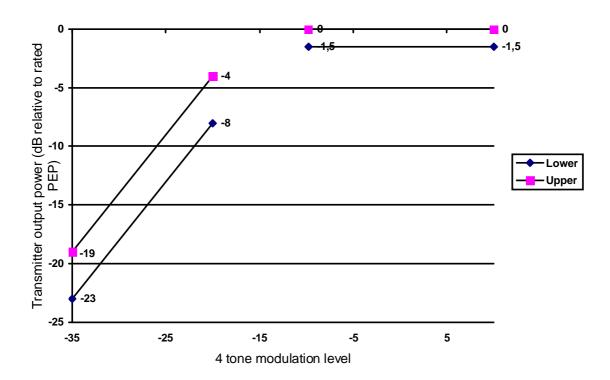
Figure 1: Limits of telephony level control
