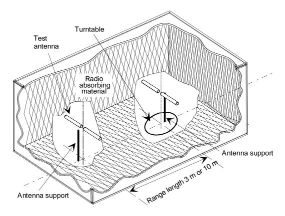
Figure A.1: A typical anechoic chamber
