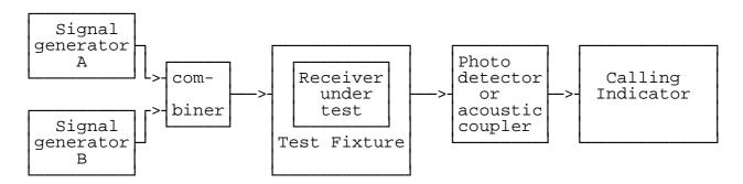
Figure 12: Measurement arrangement
