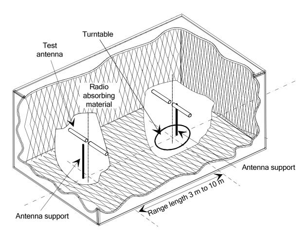
Figure A.1: A typical anechoic chamber
