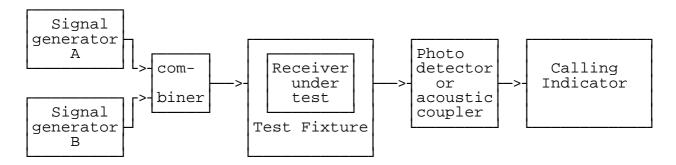
Figure 13: Measurement arrangement
