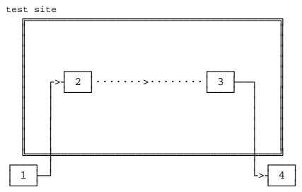
NOTE 1: Signal generator NOTE 2: Substitution antenna NOTE 3: Test antenna
