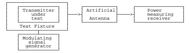
Figure 5: Measurement arrangement
