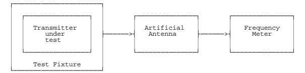
Figure 1: Measurement arrangement
