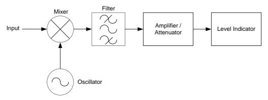
Figure B.1: Power measuring receiver
