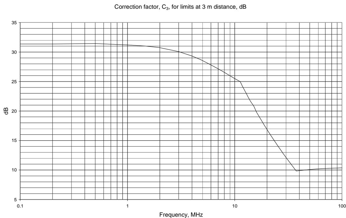
**Figure F.2: Conversion factor  $C_3$  versus frequency**
