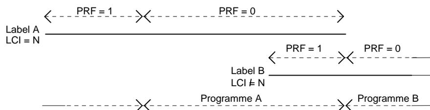
**Figure 11: PRF to signal precise start times**
