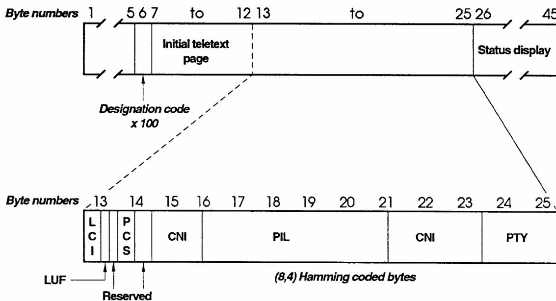
Figure 7: Structure of the Teletext data packet 8/30 format 2
