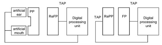
Figure 3: The direct digital processing approach test configurations for a separate PP and a separate FP
