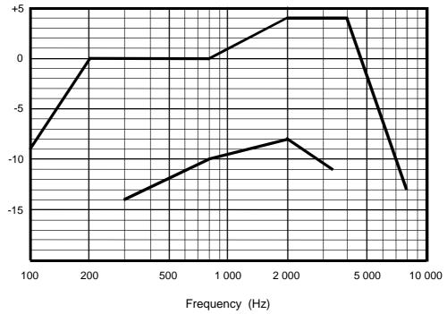
Figure 6: Sending frequency response tolerance mask
