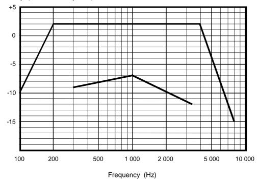
Figure 7: Receiving frequency response tolerance mask
