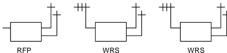
NOTE: A WRS is locked to the closest RFP, or closest WRS when cascaded WRSs are allowed. An RFP and WRS, appear equal to a PP.
