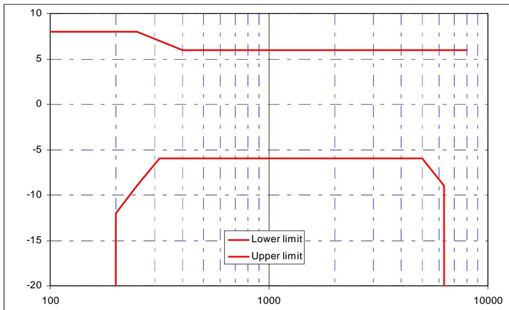
Figure 7.16: Receiving sensitivity/frequency mask for Desktop handsfree PP
