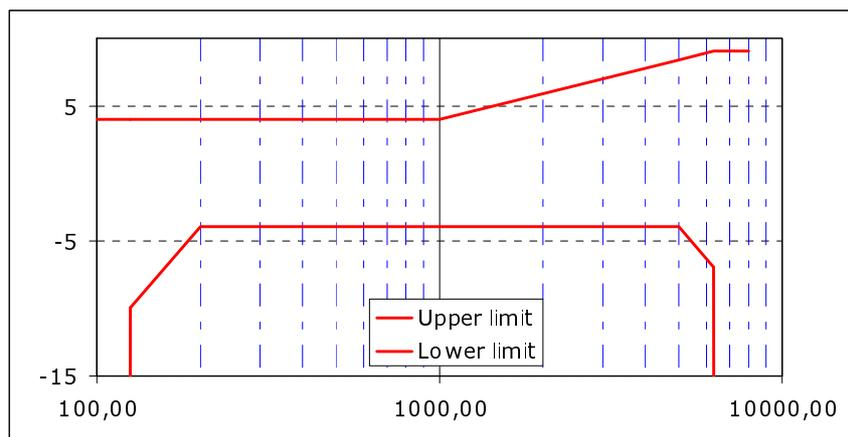
**Figure 7.15: Sending sensitivity/frequency mask for HFT**
