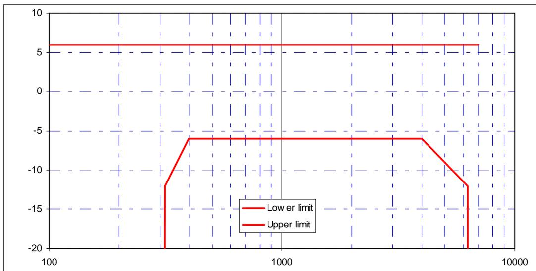
**Figure 7.17: Receiving sensitivity/frequency mask for improved handheld PP**
