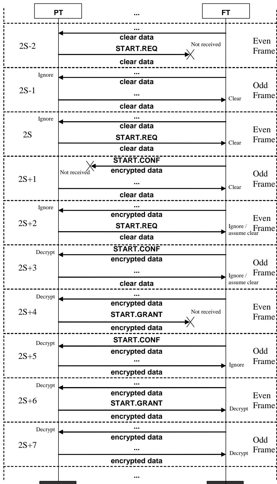
Figure 6.9: Encryption start - poor link example
