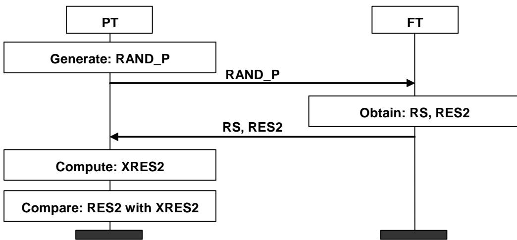
**Figure 4.2: Authentication of FT (type 1 procedure)**
