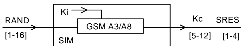
Figure G.1: Security functionality of a SIM
