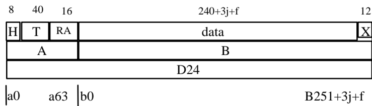
Figure 6.15 (continued): Unprotected B-field slot field structures for 4- and 8- level modulation slot formats
