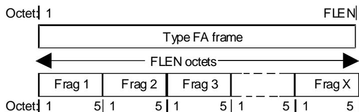
**Figure 6.1.4.2.1: C<sub>S</sub>/CL<sub>S</sub> logical channel fragmentation**
