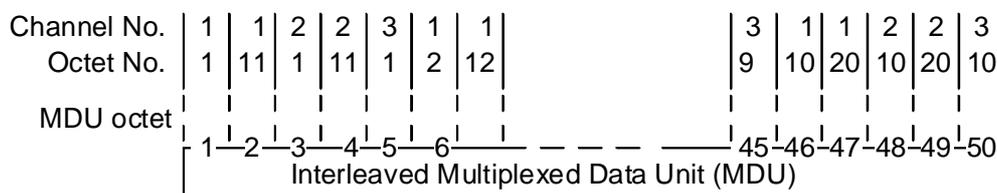
**Figure 11.6.2.3.2: Example of interleaved packing (MCS Ref: P2/16)**
