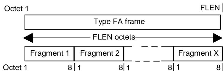
**Figure 6.1.4.1.1: C<sub>F</sub>/CL<sub>F</sub> logical channel fragmentation**
