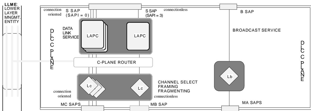
NOTE: There is one set of lower SAPs (one MA, one MB and one MC) for each instance of MAC cluster control functions (see EN 300 175-3 [3]).
