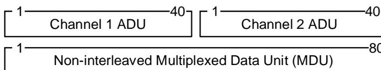
**Figure 11.6.3.3.1: Example of non-interleaved packing (MCS Ref: N2/32)**
