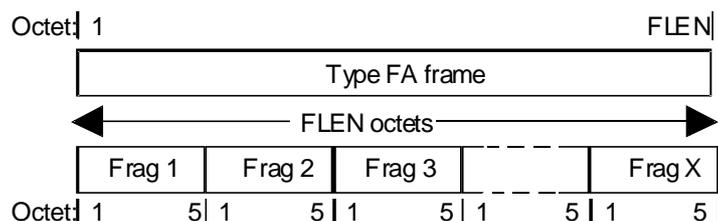
**Figure 6.1.4.2.1: C<sub>S</sub>/CL<sub>S</sub> logical channel fragmentation**
