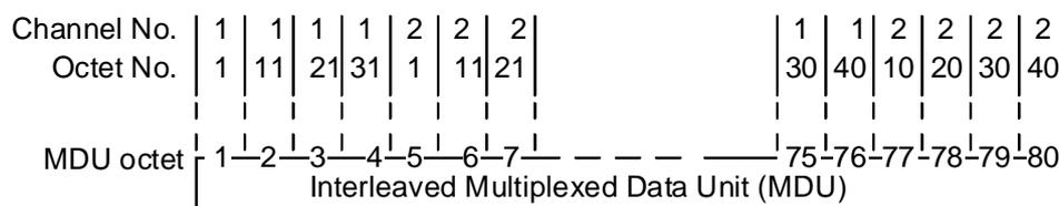
**Figure 11.6.3.3.2: Example of interleaved packing (MCS Ref: N2/32)**
