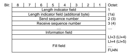
Figure 12.5.1.1: Frame format type FU4a
