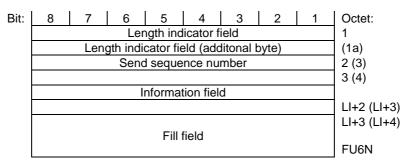
Figure 12.7.1.1: Frame format type FU6a
