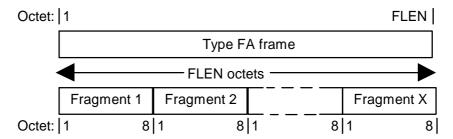
Figure 6.1.4.1.1: C<sub>E</sub>/CL<sub>E</sub> logical channel fragmentation
