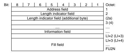
Figure 12.3.1.1: Frame Format Type FU2
