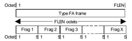
Figure 6.1.4.2.1: C<sub>S</sub>/CL<sub>S</sub> logical channel fragmentation
