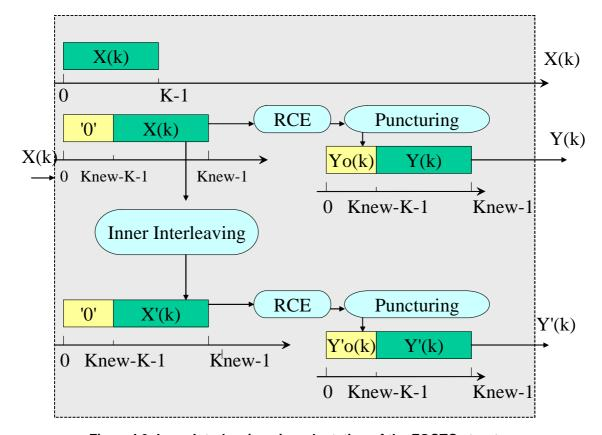
Figure I.6: Inner Interleaving size adaptation of the FOCTC structure
