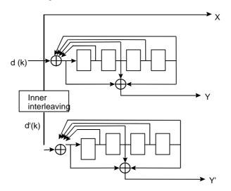
Figure I.4: FOCTC structure
