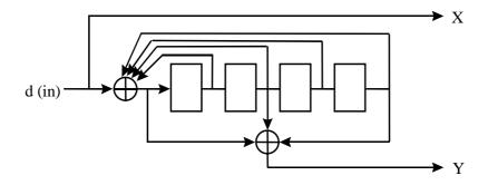
Figure I.3: Recursive Systematic Convolutional (RSC) code
