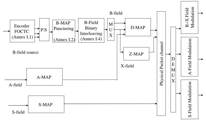
Figure I.1: B-field Channel Encoding scheme
