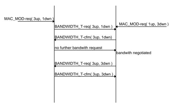
Figure 10.1: Bandwidth Modification example
