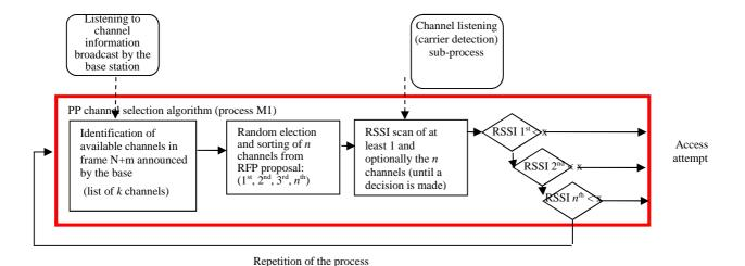
Figure 11.3: Internal diagram of Channel Selection Process M1 (PP side channel selection process)
