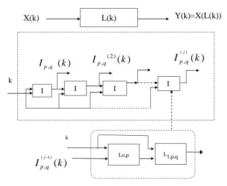
Figure I.7a: The interleaving turbo structure principle
