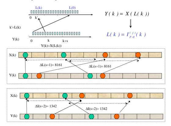
Figure I.9: Interleaving spreading definition and notations
