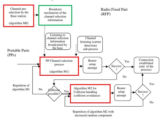
Figure 11.2: Overall architecture of ULE Channel Selection Processes
