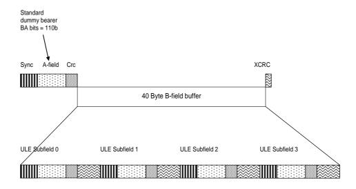
Figure 9.9: ULE Dummy Bearer showing BField data
