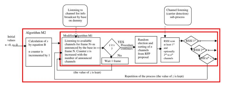
Figure 11.4: Internal diagram of Channel Selection Process M2 (PP side collision avoidance process)
