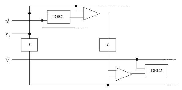
Figure J.1: Turbo Code Decoder structure
