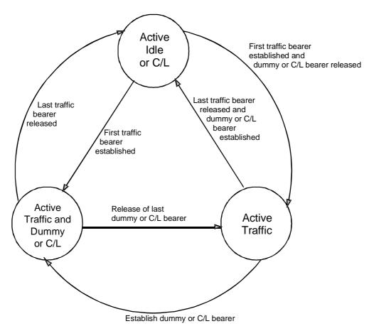
Figure 4.8: RFP state diagram
