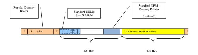
Figure 9.13b: Layout of the P00j=640 packet
