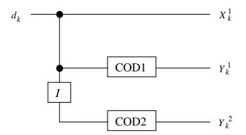
Figure I.2: Classic parallel - concatenated Turbo Code Encoder structure
