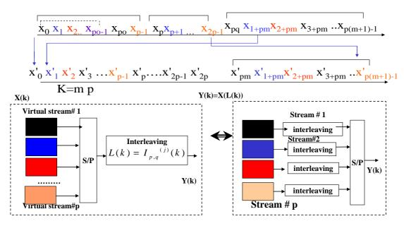
Figure I.8: The equivalent multi-stream interleaving processing
