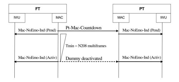
Figure 9.1: Successful activation of "no-emission" mode
