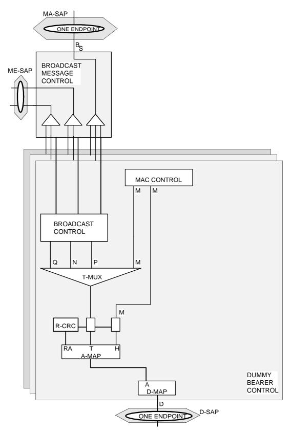
Figure 6.3: DBC multiplexing
