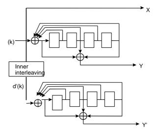
Figure I.4: FOCTC structure
