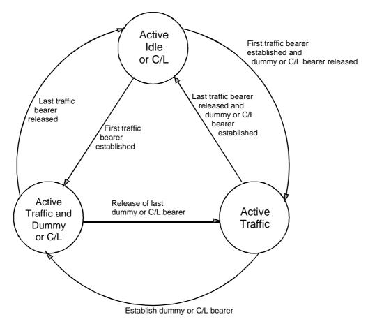
Figure 4.8: RFP state diagram
