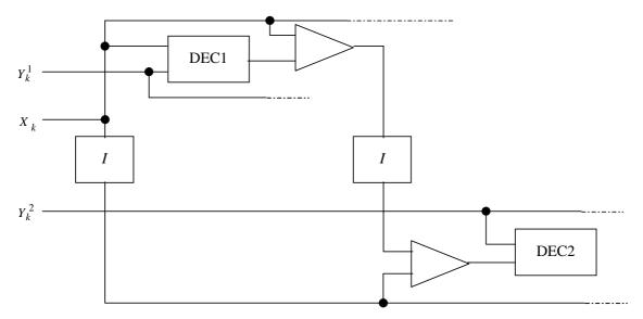
Figure J.1: Turbo Code Decoder structure
