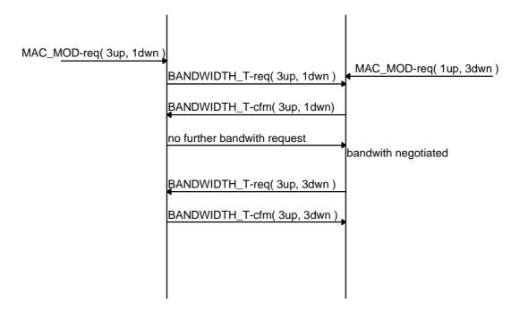
Figure 10.1: Bandwidth Modification example
