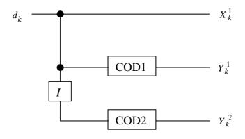
Figure I.2: Classic parallel - concatenated Turbo Code Encoder structure
