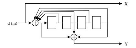
Figure I.3: Recursive Systematic Convolutional (RSC) code
