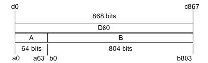
Figure 6.5: A-field and B-field in the D80 field (double slot, 2 level modulation)
