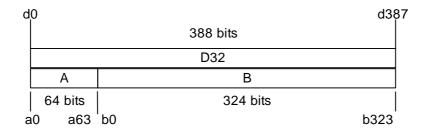
Figure 6.8: A-field and B-field in the D32 field (full slot, 2 level modulation)
