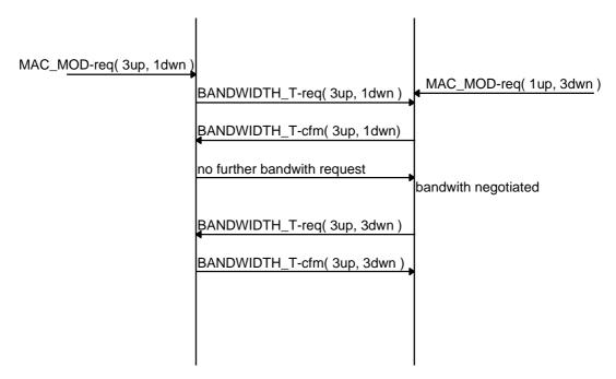
Figure 10.1: Bandwith Modification example
