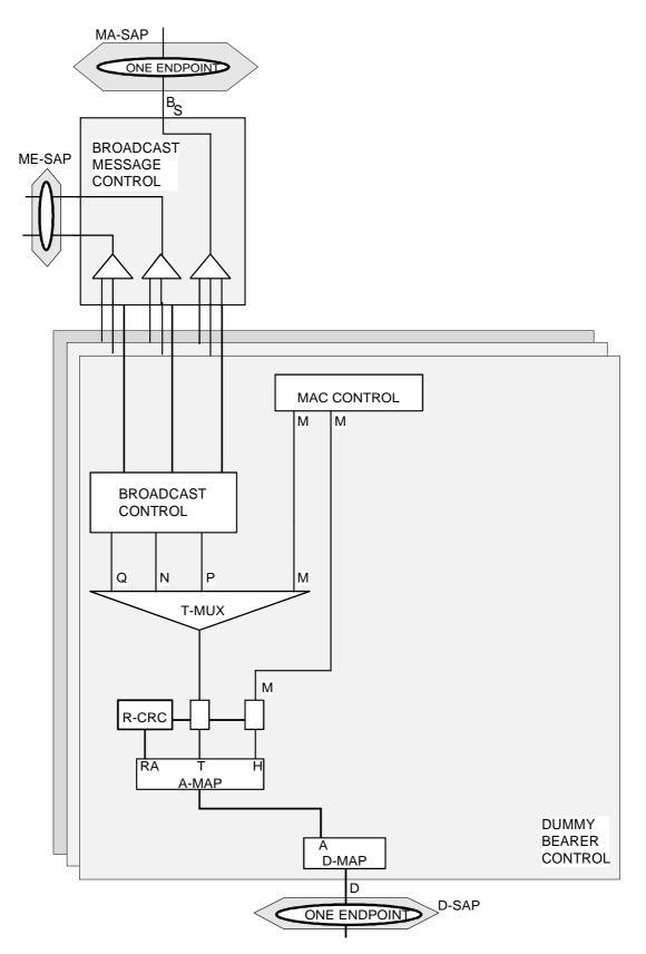
Figure 6.3: DBC multiplexing
