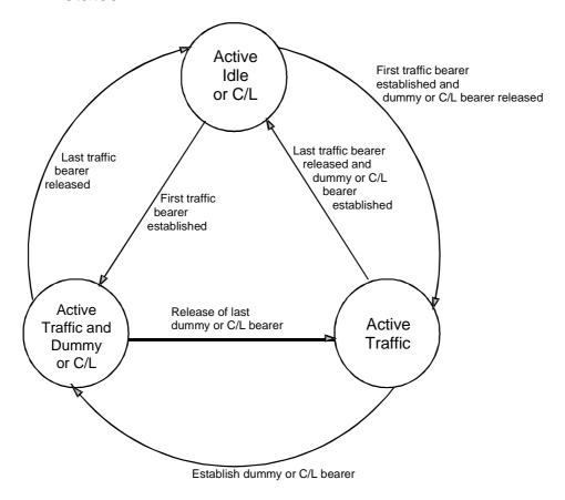
Figure 4.8: RFP state diagram
