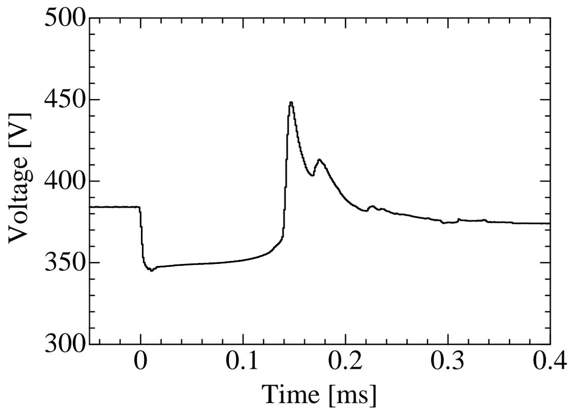
Figure G.3: Example of result of short circuit and voltage transient measurement on simulation circuit described in figure G.2
