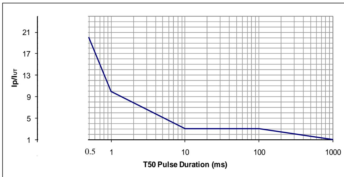
Figure 3: Maximum inrush current characteristics for telecommunications and datacom (ICT) equipment > 250 W at  $U_T$
