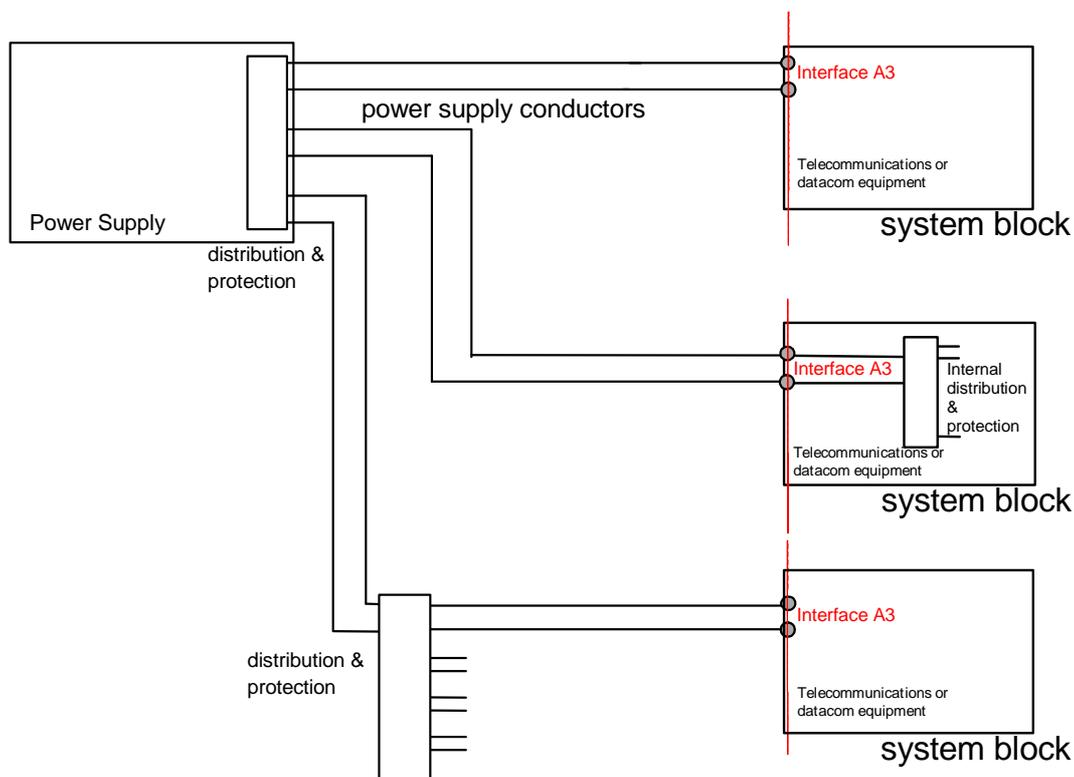
NOTE 1: The figure is a drawing of the power system and does not show the PE conductor.
