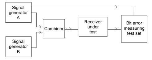
Figure 28: Measurement arrangement
