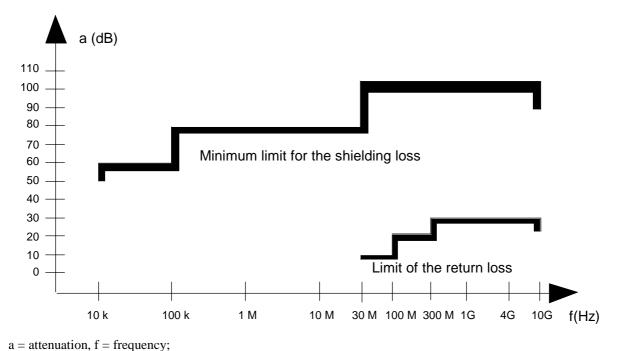
Figure A.3: Specifications for shielding and reflections
