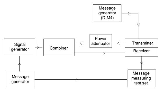
Figure 36: Measurement arrangement
