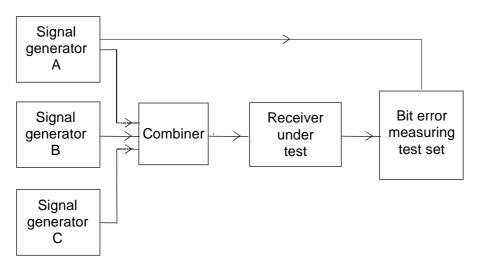
Figure 26: Measurement arrangement
