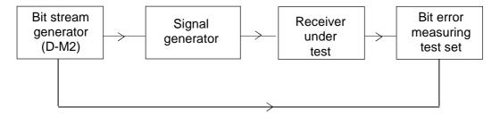
Figure 19: Measurement arrangement
