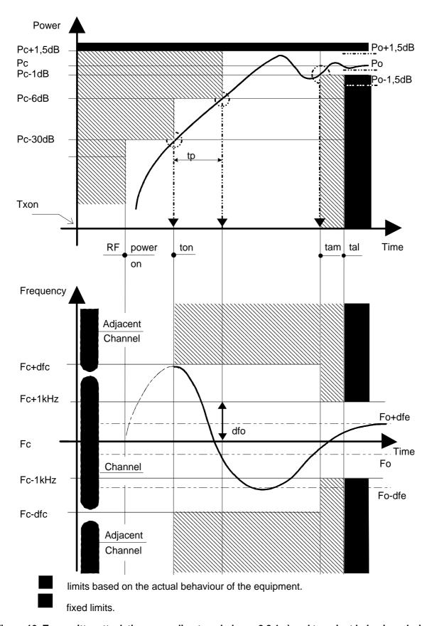
Figure 12: Transmitter attack time according to subclause 8.8.1 a) and transient behaviour during switch-on. (Case where the attack time is given by the behaviour of the power rise)
