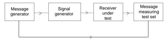
Figure 18: Measurement arrangement
