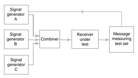
Figure 27: Measurement arrangement
