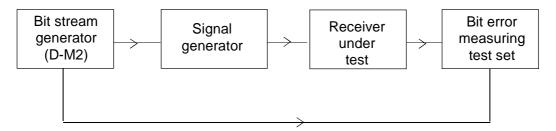
Figure 17: Measurement arrangement
