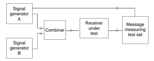
Figure 24: Measurement arrangement
