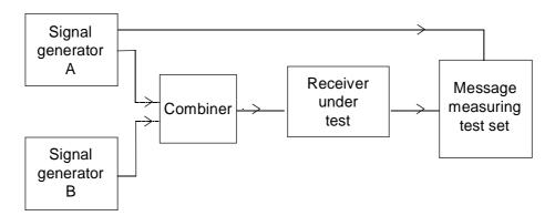
Figure 29: Measurement arrangement
