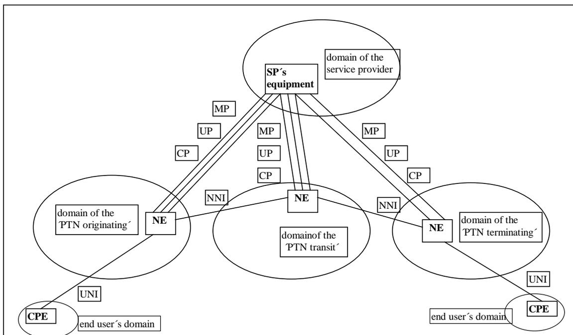
**Figure 47: Location of the control-, user-, and management-related functions between the equipment of an SP and PTNs**
