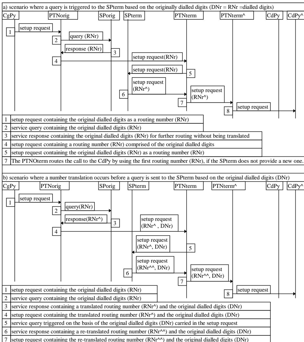
**Figure 35: Reception of the originally dialled digits**
