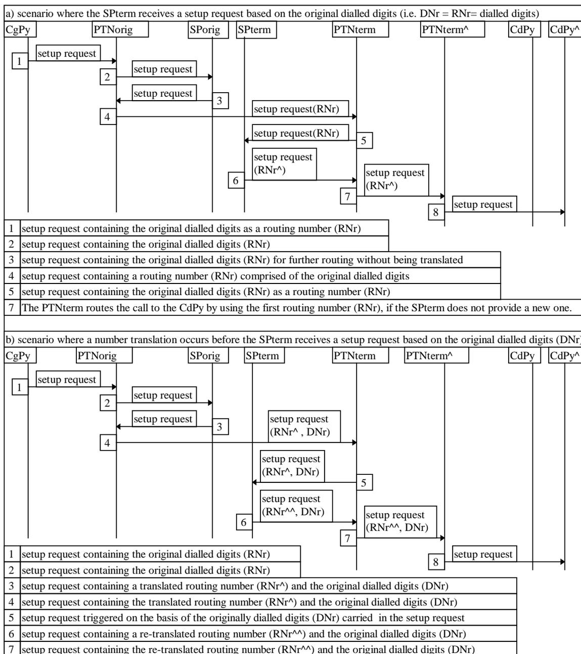
**Figure 15: Reception of the originally dialled digits**
