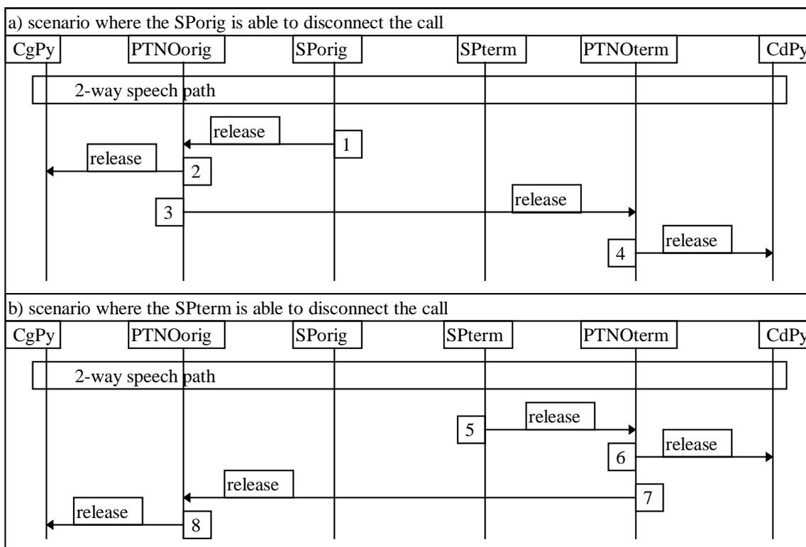
Figure 16: Disconnection of a call in progress
