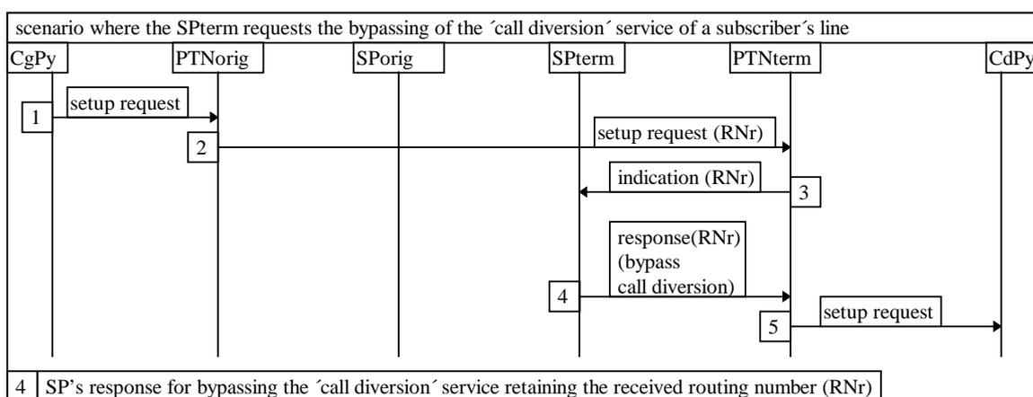
**Figure 41: Bypassing of the "call diversion" supplementary service**
