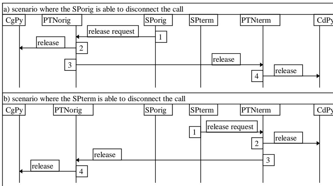
**Figure 36: Disconnection of a call in progress**
