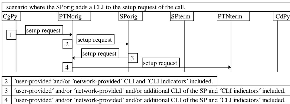
**Figure 4: Addition of a calling line identity**
