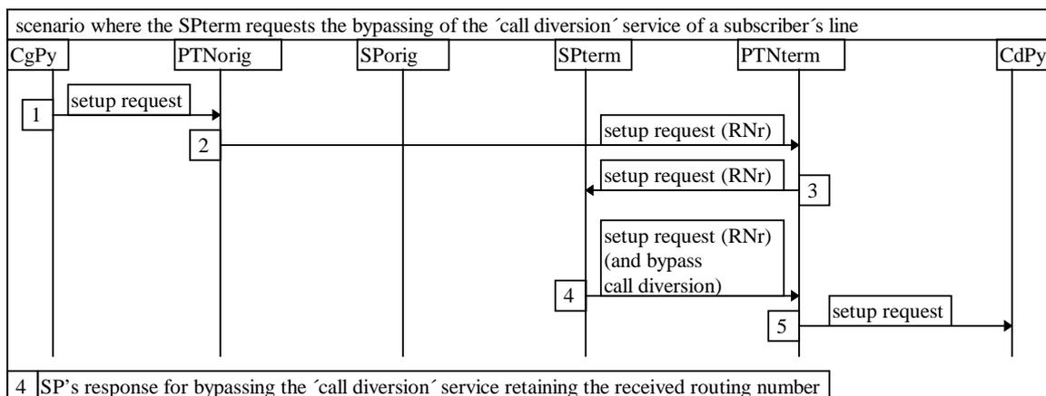
**Figure 20: Bypassing of the call diversion supplementary service**
