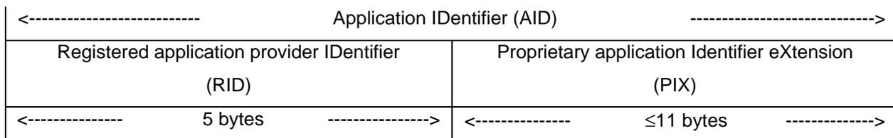
The AID consists of a Registered application provider IDentifier (RID) of 5 bytes and a Proprietary application Identifier eXtension (PIX) of up to 11 bytes.
