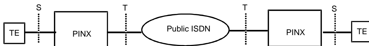
Figure 7: CN TE to CN TE via public ISDN
