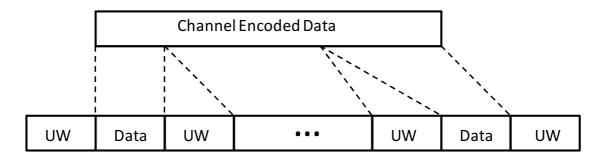
Figure 7-17: CC-CPM burst structure
