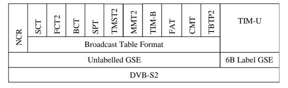
Figure 6-1: Protocol Stack for Lower Layer Signalling over a Continuous Generic Stream Forward Link
