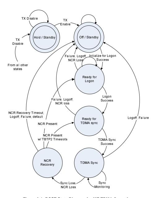
Figure 9-1: RCST State Diagram for MF-TDMA Operation
