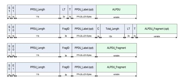
Figure 7-2: Payload-adapted PDU Formats
