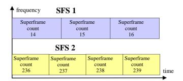
Figure 7-24: Example of superframe sequences
