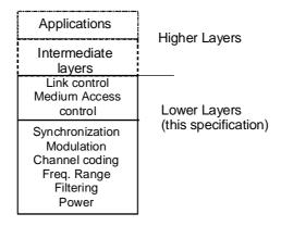
Figure 4-1: Identification of the Lower Layers
