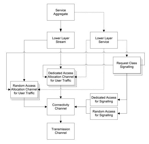
Figure 4-3: Mapping of a Service Aggregate in the Lower Layers
