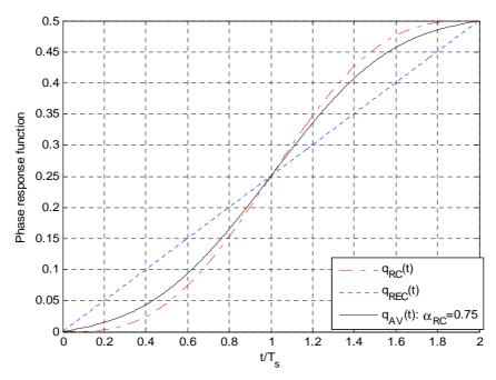
Figure 7-20: Phase response for RC, REC and AV pulse shapes
