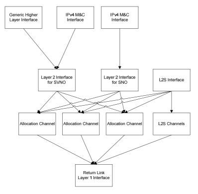
Figure 4-6: Return Link Interfaces at an RCST
