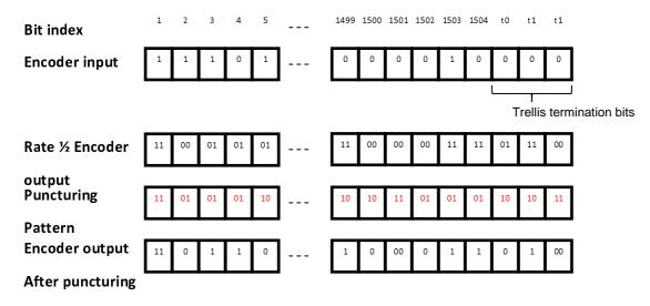
Figure 7-15: Puncturing process for rate 6/7, K=4 convolutional code
