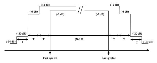
Figure 7-21: Burst power envelope mask for TC-LM bursts
