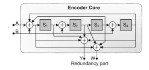
Figure 7-11: Encoder block diagram (turbo code)
