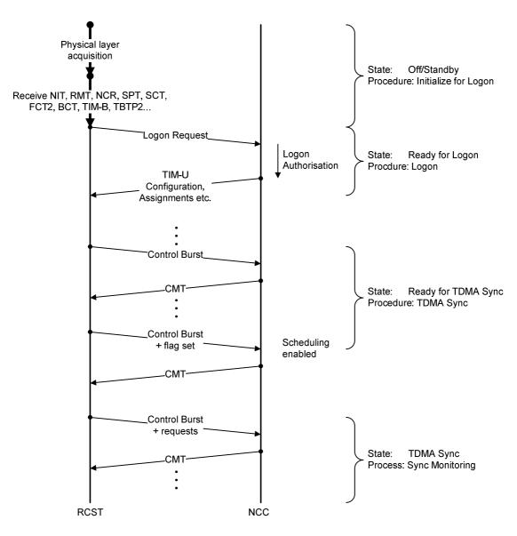
Figure 9-2: Example of Interactive Network Lower Layer Signalling Flow on the FL, the SFS to be Used for Logon and the SFS to be Used for Operation
