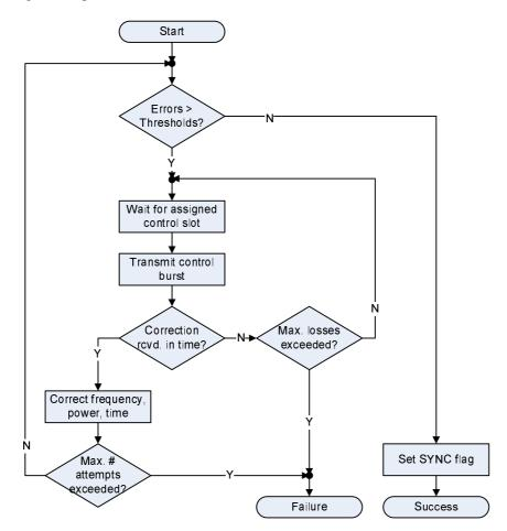
Figure 9-4: TDMA Synchronization Procedure
