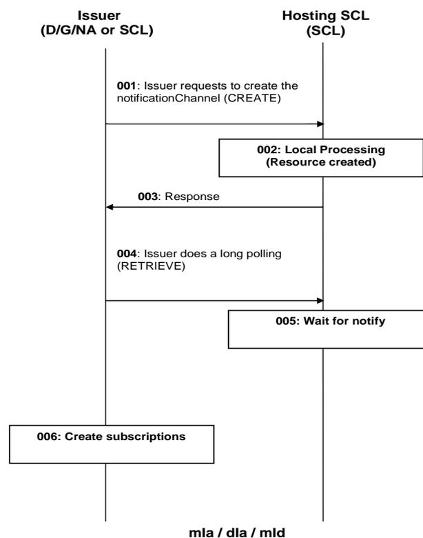
**Figure 9.113: Procedures for *<notificationChannel>* create**
