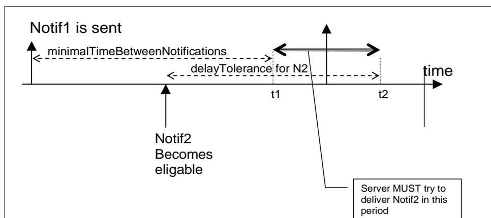
**Figure 9.86: Notification mechanism, no conflict between the subscription minimalTimeBetweenNotification and the resource instance delayTolerance**
