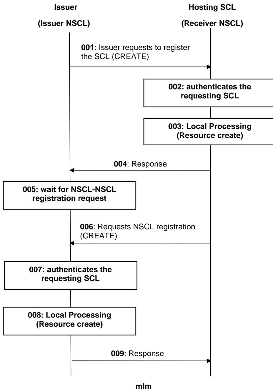
**Figure 9.51a: Procedures for NSCL to NSCL registration over mlm (for Inter-domain communication)**
