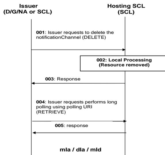
**Figure 9.115: Procedures for <notificationChannel> delete**
