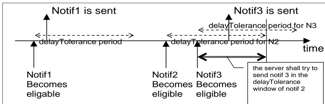
**Figure 9.84: Notification mechanism, conflict resolution when multiple delayTolerance are used**
