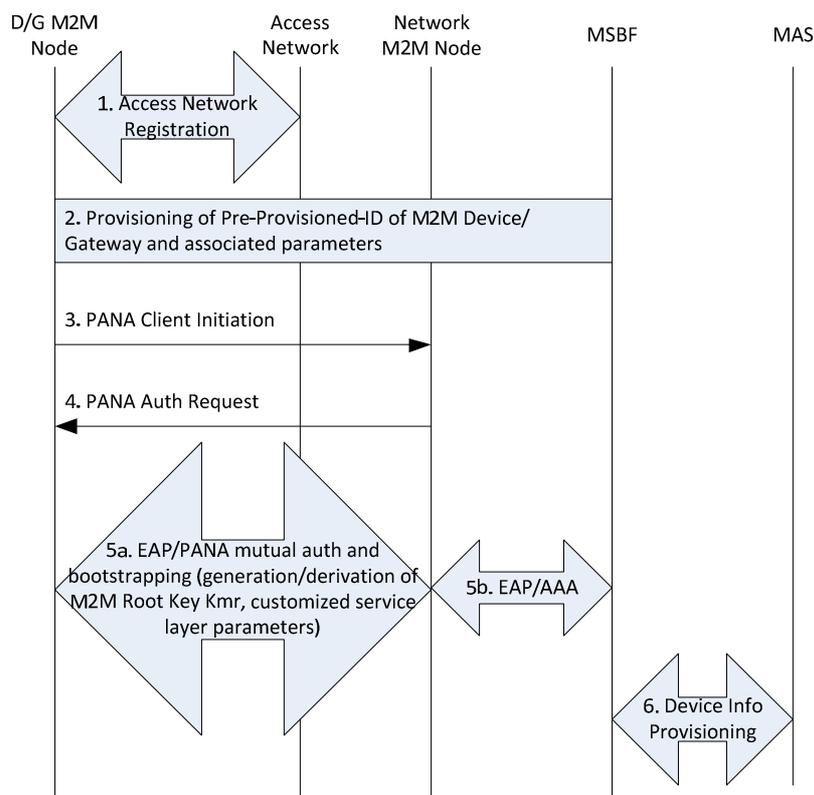
**Figure 8.6: M2M Service Bootstrap using automated method**
