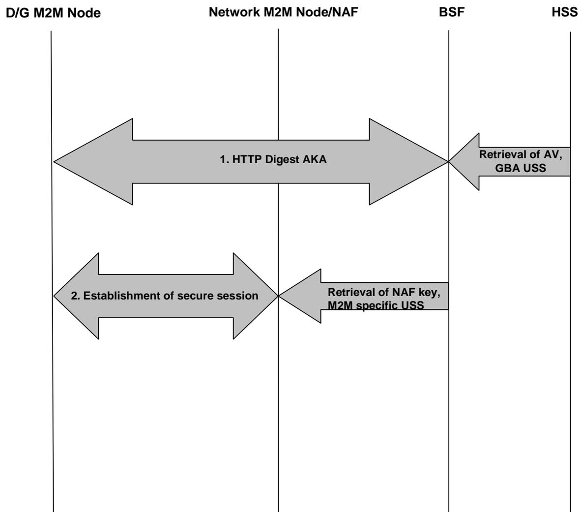
**Figure 8.13: M2M Service Connection procedure based on GBA**
