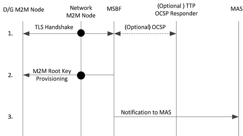
**Figure 8.9: Call flow for Automated Bootstrapping using Device-Certificate TLS over TCP**
