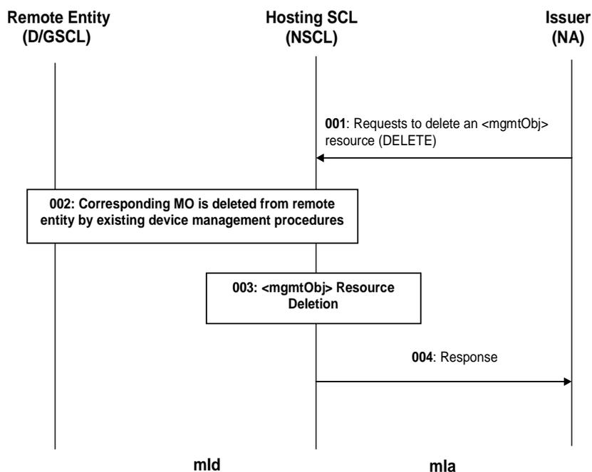
**Figure 9.101: Illustration of procedures to delete an <mgmtObj> resource by NA**
