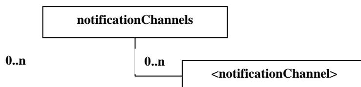
**Figure 9.34: Structure of notificationChannels resource**
