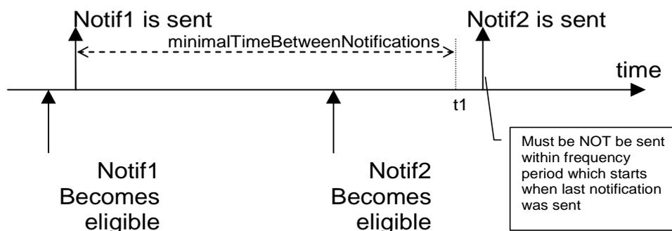
**Figure 9.81: Notification mechanism when minimalTimeBetweenNotifications is used**
