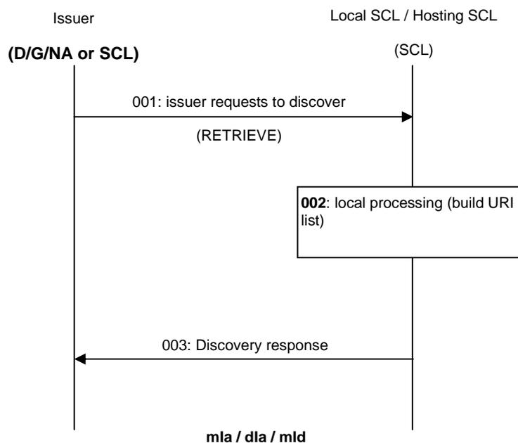
**Figure 9.117: Discovery procedure message flow**
