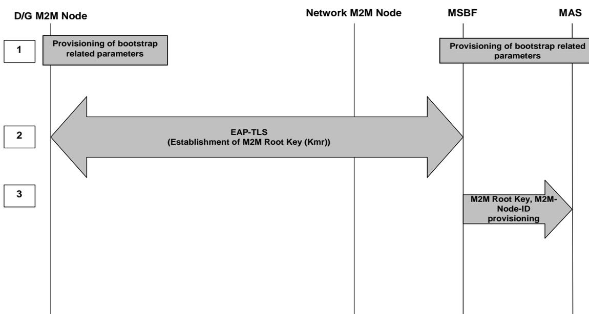
**Figure 8.8: M2M Service Bootstrap using EAP-TLS over PANA**
