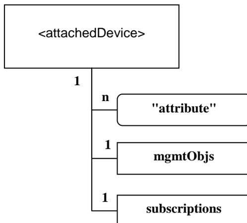
**Figure 9.33: Structure of <attachedDevice> resource**
