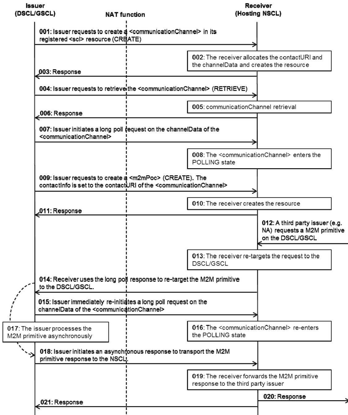
**Figure H.4: Message flow to handle the NAT traversal on mld (server layer option)**
