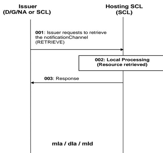
**Figure 9.114: Procedures for *<notificationChannel>* retrieve**
