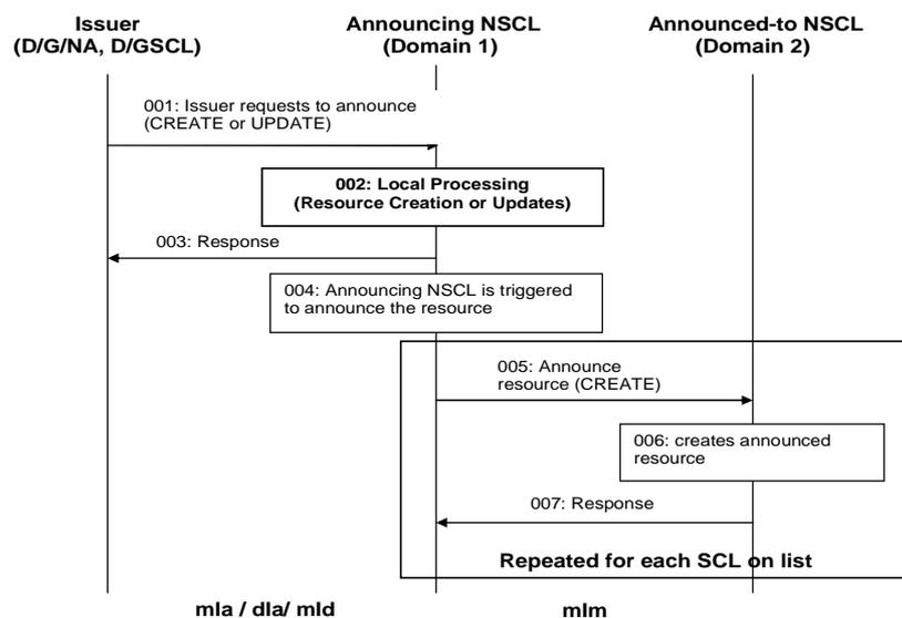
**Figure 9.119a: Illustration of Procedures to Announce Resources w/ immediate Response over mIm**
