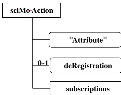
**Figure B.2: Structure of the scIMoAction resource**
