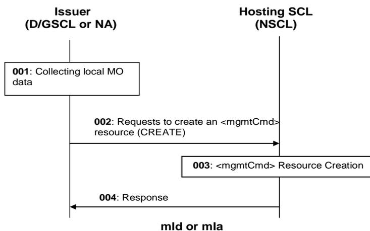
**Figure 9.104: Illustration of procedures to create an *<mgmtCmd>* resource by D/GSCL**
