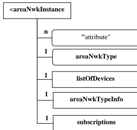
Figure B.27: Structure of the &lt;areaNwkInstance&gt; resource
