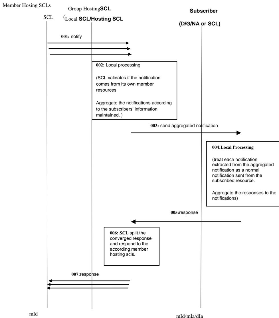
**Figure 9.76a: Illustration of Procedures to Verify Membership**
