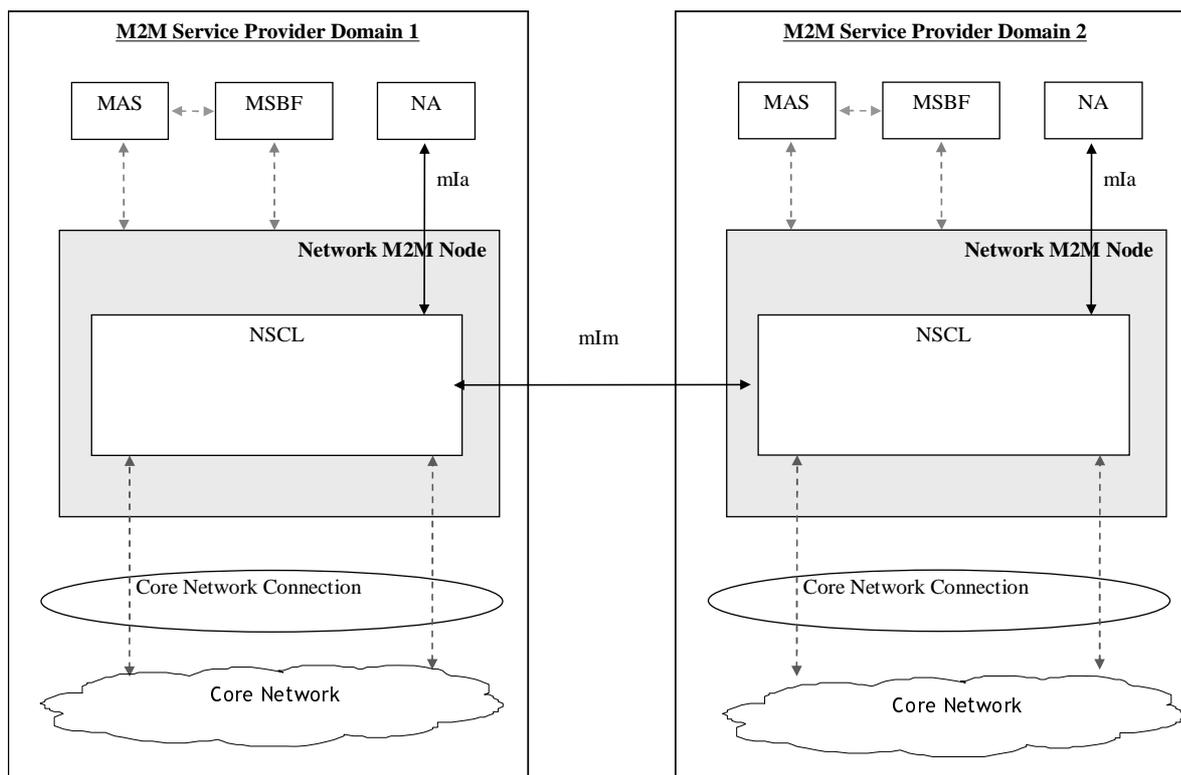
**Figure 5.1a: Inter-M2M Service Provider functional architecture framework**
