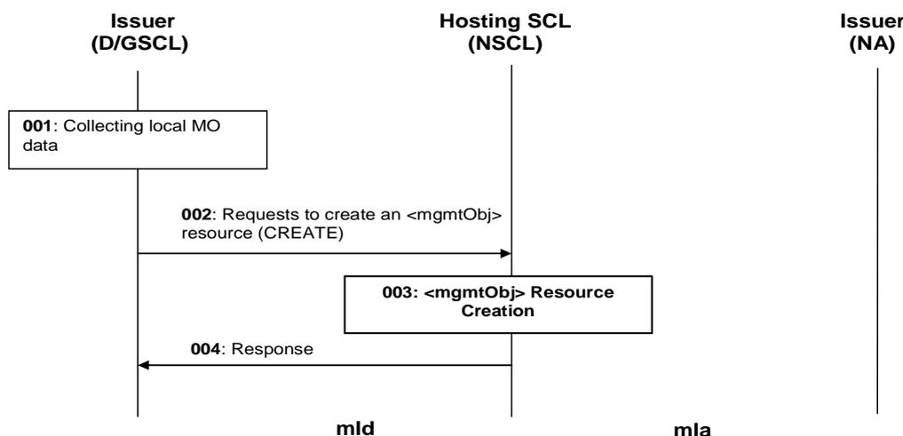
**Figure 9.94: Illustration of procedures to create an *<mgmtObj>* resource by D/GSCL**
