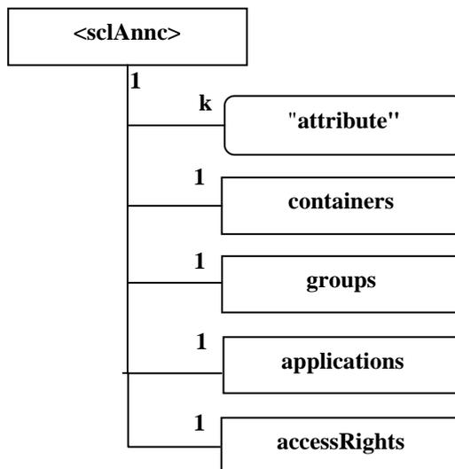
**Figure 9.39: Structure of  $\langle \text{sclAnnC} \rangle$  resource**
