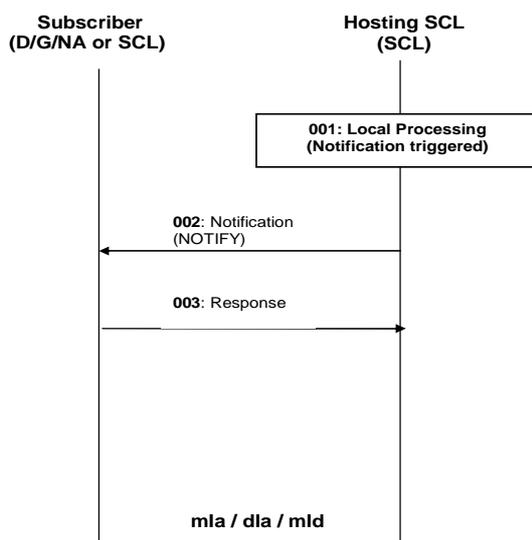
**Figure 9.88: Procedures for asynchronous notification**
