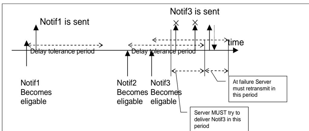
**Figure 9.85: Notification mechanism, the case of failure to transmit notifications on time**
