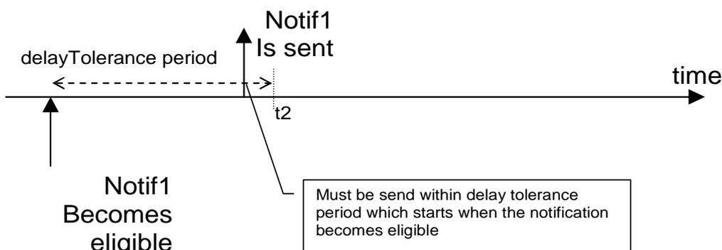
**Figure 9.83: Notification mechanism when `delayTolerance` is used**
