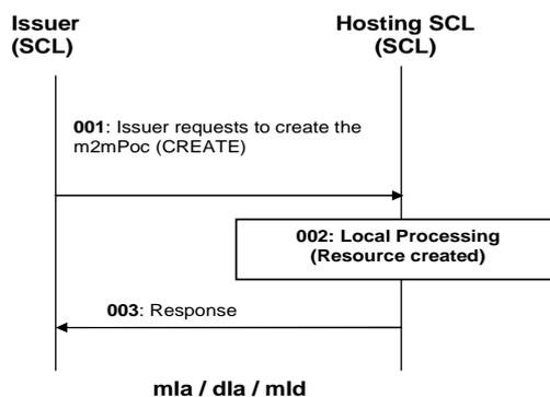
**Figure 9.90: Procedures for <m2mPoc> create**
