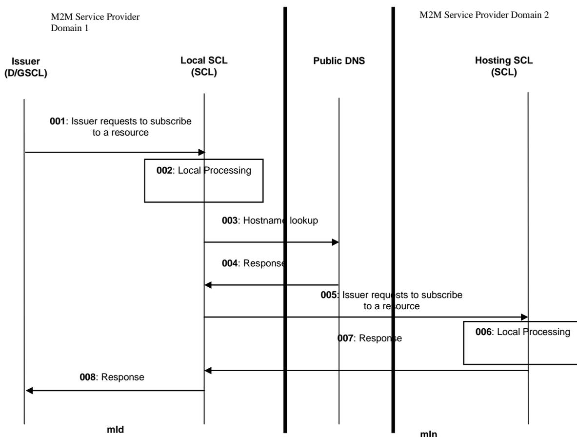
**Figure 9.131: Message flow of procedure to subscribe to a resource in another M2M Service Provider domain**
