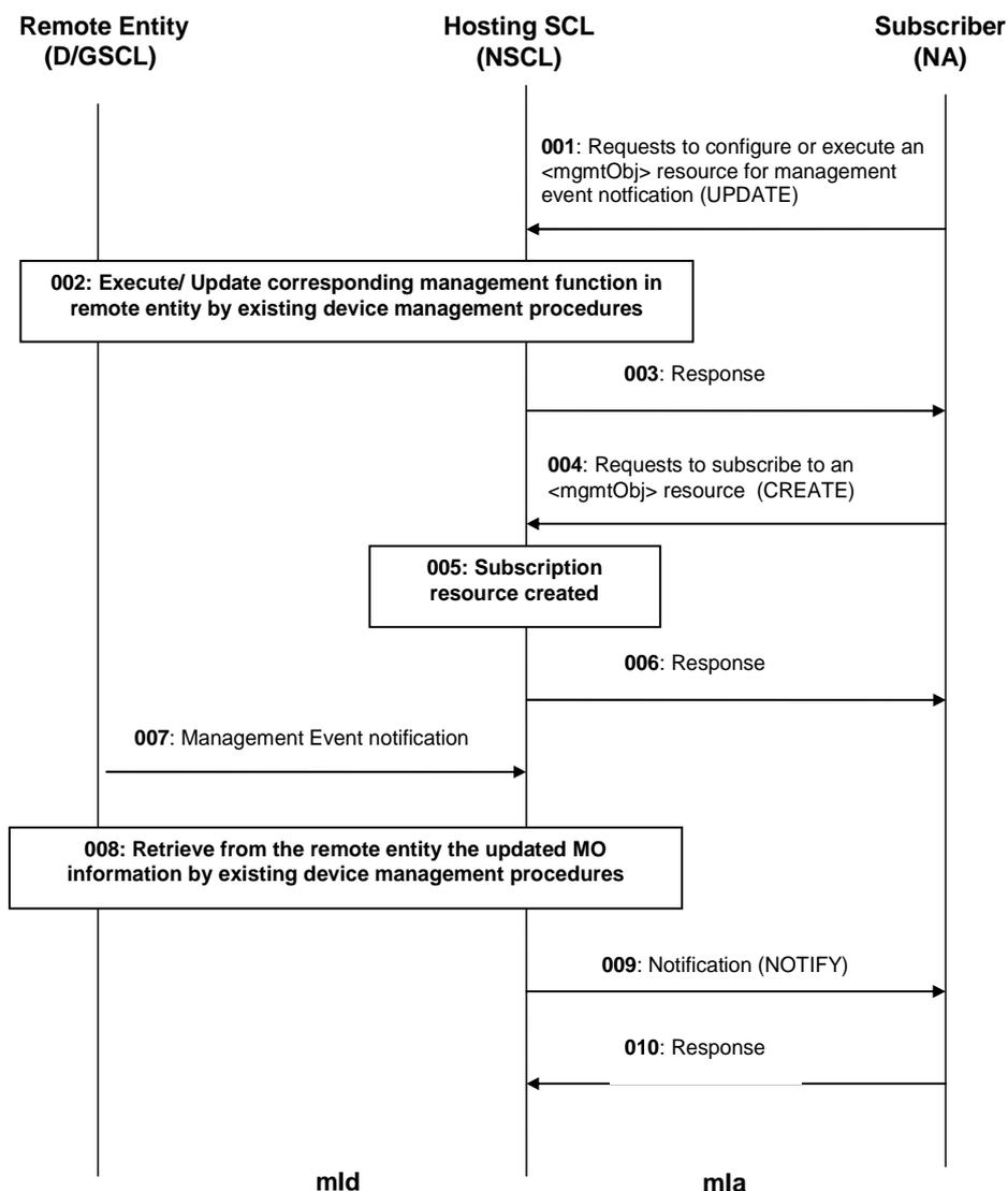
**Figure 9.103: Illustration of procedures to subscribe/notify an <mgmtObj> resource**
