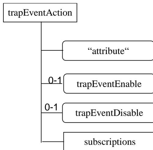
**Figure B.15: Structure of the trapEventAction resource**
