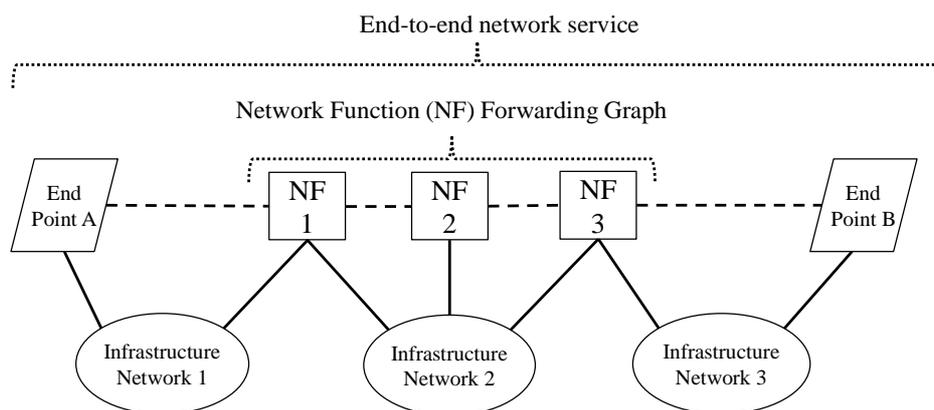
**Figure 2: Graph representation of an end-to-end network service**
